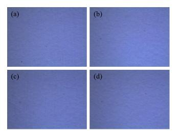
**Figure 2.** Outer layers surface of samples analyzed under a stereomicroscope with  $10 \times$  magnification. (a,c) control, (b,d) aqueous food simulant processed by ultrasound for 60 min, (a,b) Film A and (c,d) Film B.
