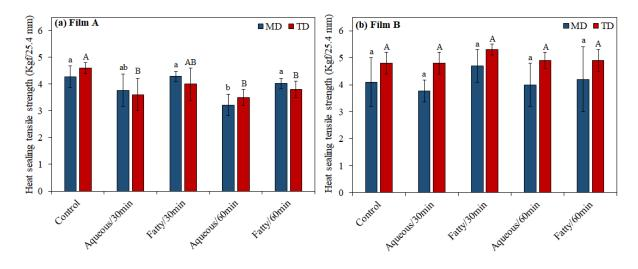
**Figure 7.** Heat sealing tensile strength of different packaging materials processed by ultrasound. (a) Film A: PE/PA/PE, (b) Film B: PE/PA/PE/PA/PE, MD: machine direction and TD: transverse direction.
