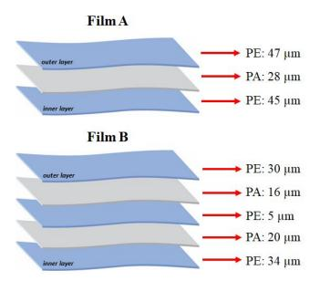
Figure 1. Composition of PE and PA multilayer films and their respective thicknesses.
