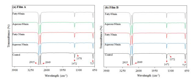
**Figure 3.** FT-IR spectra of inner layer of different packaging materials processed by ultrasound. (a) Film A: PE/PA/PE and (b) Film B: PE/PA/PE/PA/PE.
