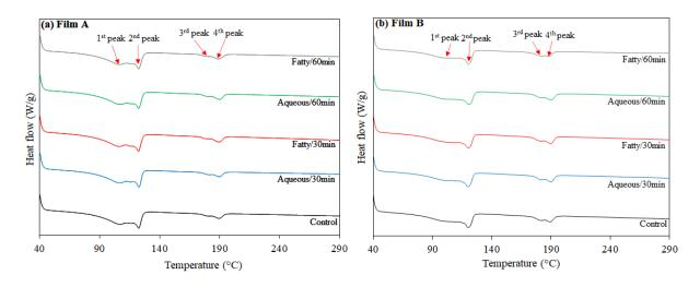
**Figure 5.** Differential Scanning Calorimetry of different packaging materials processed by ultrasound. (a) Film A: PE/PA/PE and (b) Film B: PE/PA/PE/PA/PE.
