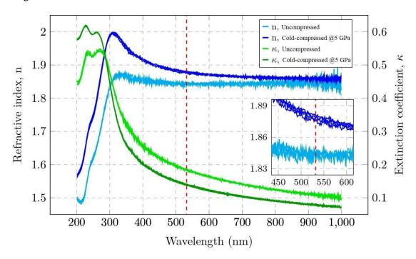
Figure 4: Real part (n) and extinction coefficient (K) of the refractive index, obtained at 55°, 60°, and 65°, for the Belt cold-compressed at 5 GPa and uncompressed PS samples obtained upon direct inversion. The dashed line at  $\lambda$ =532 nm marks the Brillouin probing wavelength with the respective n values zoomed in the inset.
