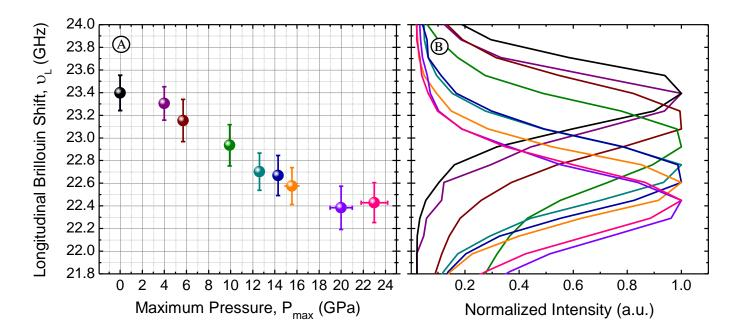
Figure 3: (a) Longitudinal Brillouin line shift ( $v_L$ ) as a function of the maximum pressure ( $P_{max}$ ) and (b) Brillouin spectra of the uncompressed and cold densified PS samples. Brillouin measurements were recorded at atmospheric pressure after a complete compression-decompression cycle in the DAC apparatus. Uncertainties in the Brillouin values were evaluated as one-eighth of the related line width.
