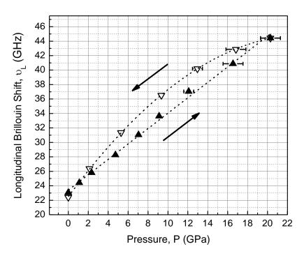
Figure 2: In-situ longitudinal Brillouin line shift  $(v_L)$  of PS glass up to 20 GPa in a complete compression and decompression cycle in the DAC.
