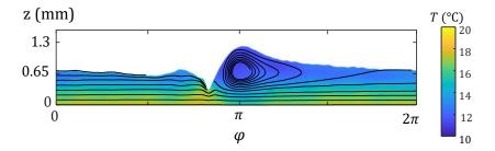
Figure A.1: Stream lines of the flow in the liquid film under a wave obtained using the Kapitza-Shkadov model used for the velocity calculation, printed over the temperature field measured by PLIF. Results for Re = 200,  $\beta = 10^{\circ}$ , f = 10 Hz, x = 160 mm,  $T_i = 10^{\circ}$ C and  $q_w = 1.25$  W/cm<sup>2</sup>
