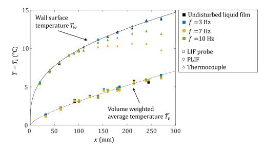
Figure 10: Spatial evolution of the volume weighted average temperature of the liquid film  $T_v$  and  $T_w$  the wall surface temperature. Comparison to the theoretical model for the undisturbed flat liquid film in dotted and solid lines respectively, with Re = 200,  $\beta = 10^{\circ}$  and  $q_w = 1.25 \text{ W/cm}^2$ .
