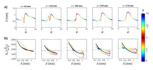
Figure 21: Evolution of the thickness  $\delta$  (a) and the heat transfer coefficient  $h_v$  (b) of the falling liquid film compared to the pure diffusion model (black line). The color of the curves is matched in phase between the two rows. The horizontal dotted line is the time average heat transfer coefficient calculated from the experimental data from the LIF probe. Results for f = 7 Hz, Re = 200,  $\beta = 10^{\circ}$ ,  $T_i = 10^{\circ}$ C and  $q_w = 1.25 \text{ W/cm}^2$ .
