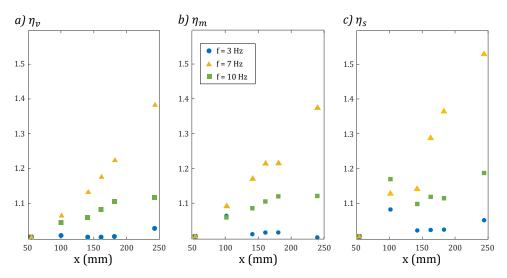
Figure 13: Spatial evolution of the efficiency factor  $\eta$  calculated with the three previously defined film temperature  $T_m$ ,  $T_v$  and  $T_s$ . Same experimental conditions as in Fig. 12. As in Fig. 12, the points at x = 50 mm were hand placed to help read the trends.
