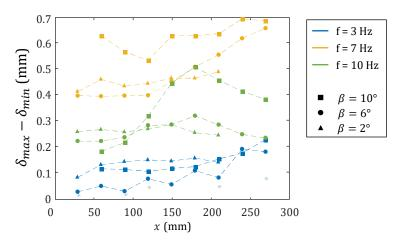
Figure 9: Spatial evolution of the amplitude of the waves for three perturbation frequency f = 3 Hz, f = 7 Hz and f = 10 Hz represented along the flow distance x. The measurements are represented for Re = 200 and  $q_w = 1.25$  W/cm<sup>2</sup>. The dotted curves were hand drawn to help reading.
