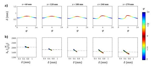
Figure 20: Evolution of the thickness  $\delta$  (a) and the heat transfer coefficient  $h_v$  (b) of the falling liquid film compared to the pure diffusion model (black line). The color of the curves is matched in phase between the two rows. The horizontal dotted line is the time average heat transfer coefficient calculated from the experimental data from the LIF probe. Results for f = 3 Hz, Re = 200,  $\beta = 10^{\circ}$ ,  $T_i = 10^{\circ}$ C and  $q_w = 1.25$  W/cm<sup>2</sup>.
