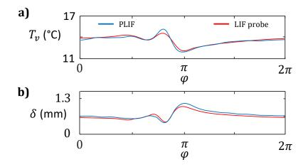
Figure 6: Comparison of the average temperature  $T_v$  (a) and the film height  $\delta$  (b) measured with the PLIF technique and the LIF probe (Re = 200,  $\beta = 10^\circ$ , x = 160 mm, f = 10 Hz,  $T_i = 10^\circ$ C and  $q_w = 1.25$  W/cm<sup>2</sup>).
