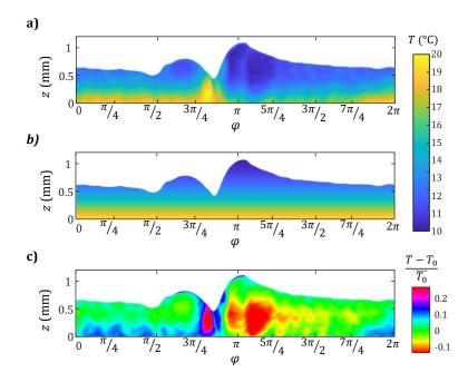
Figure 17: Temperature field T in the film obtained using PLIF measurement technique (a) and the corresponding temperature field  $T_{Nu}$  calculated with the extrapolated Nusselt solution under the assumption of pure diffusion in the transverse direction (b). The normalized difference between Tand  $T_{Nu}$  is shown in (c). Results correspond to Re = 200,  $\beta = 10^{\circ}$ , x = 180 mm, f = 10 Hz and  $T_i = 10^{\circ}$ C.
