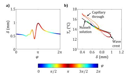
Figure 19: Evolution of the thickness  $\delta$  (a) and the volume average temperature  $T_v$  (b) during the period of a wave. The conditions correspond to f = 10 Hz, Re = 200,  $\beta = 10^{\circ}$ ,  $T_i = 10^{\circ}$ C and  $q_w = 1.25$  W/cm<sup>2</sup> and x = 180 mm. The black curve is for the theoretical model based on the Nusselt solution which allows to determine the average temperature in the film cross-section in the absence of mixing by the wave.
