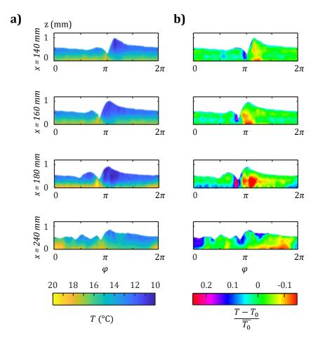
Figure 18: Spatial evolution of the temperature field T (a) and of the normalized difference between T and  $T_{Nu}$  (b) along the flow of the film. Results were obtained for Re = 200,  $\beta = 10^{\circ}$ , f = 10 Hz and  $T_i = 10^{\circ}$ C.
