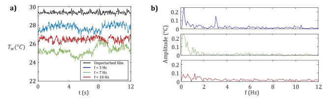
Figure 7: Variations in wall temperature during the passage of waves at different frequencies measured with Re = 200,  $\beta = 10^{\circ}$ , x = 250 mm,  $T_i = 15 \text{ °C}$  and  $q_w = 1.25 \text{ W/cm}^2$ . Raw data are presented in (a) and their corresponding FFT are presented in (b). The difference in wall temperature between the different cases is a consequence of heat transfer.
