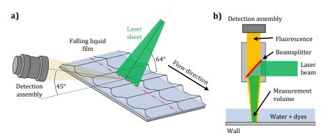
Figure 5: Optical configuration used for the LIF techniques applied to the falling film. a) Illumination by a laser sheet and detection by a camera assembly for the PLIF technique. b) Illumination and detection by the punctual LIF probe.
