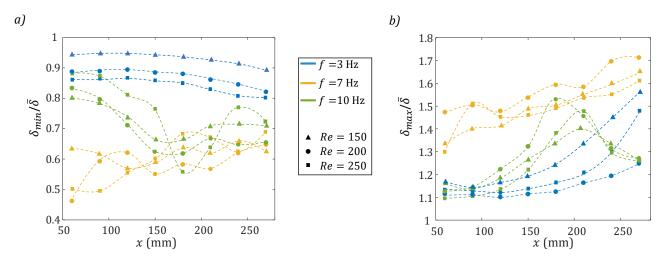
Figure 8: Evolutions of the minimum (a) and maximum (b) of the film thickness as a function of the distance x from the flow inlet. Measurements obtained with the LIF probe for three values of the Reynolds number: Re = 150 ( $\triangle$ ), Re = 200 ( $\bigcirc$ ) and Re = 250 ( $\square$ ), and  $\beta = 10$  °,  $T_i = 10$  °C and  $q_w = 1.25$  W/cm<sup>2</sup>. The dotted curves were hand drawn to help reading.
