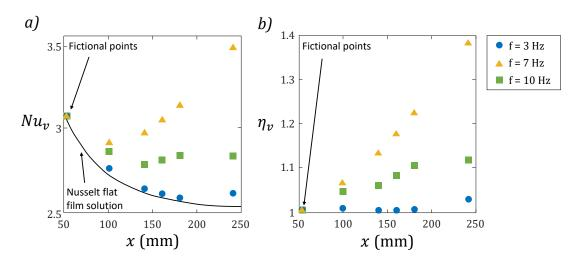
Figure 12: Spatial evolution of the Nusselt number  $\overline{\text{Nu}_v}$  (a) and  $\eta_v$  (b) along the liquid film for three perturbation frequencies f for Re = 200,  $\beta = 10^{\circ}$  and  $q_w = 1.25 \text{ W/cm}^2$ . The black line represents the Nusselt flat film solution.
