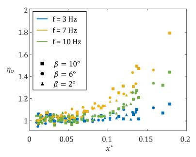
Figure 16: Evolution of the efficiency factor  $\eta_v$  obtained experimentally with the dimensionless distance  $x^*$ . The data covers the totality of the studied Re,  $\beta$  and f values.
