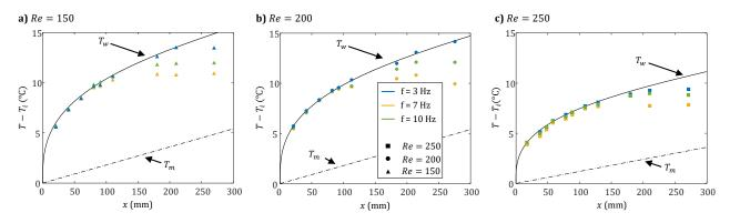
Figure 14: Spatial evolution of the measured wall temperature  $T_w$  for three Reynolds numbers Re = 150 (a), Re = 200 (b) and Re = 250 (c) and three perturbation frequencies f = 3 Hz, 5 Hz and 10 Hz,  $\beta = 10^{\circ}$  and  $q_w = 1.25$  W/cm<sup>2</sup>.
