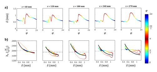
Figure 21: Evolution of the thickness  $\delta$  (a) and the heat transfer coefficient  $h_v$  (b) of the falling liquid film compared to the pure diffusion model (black line). The color of the curves is matched in phase between the two rows. The horizontal dotted line is the time average heat transfer coefficient calculated from the experimental data from the LIF probe. Results for f = 7 Hz, Re = 200,  $\beta = 10^{\circ}$ ,  $T_i = 10^{\circ}$ C and  $q_w = 1.25$  W/cm<sup>2</sup>.
