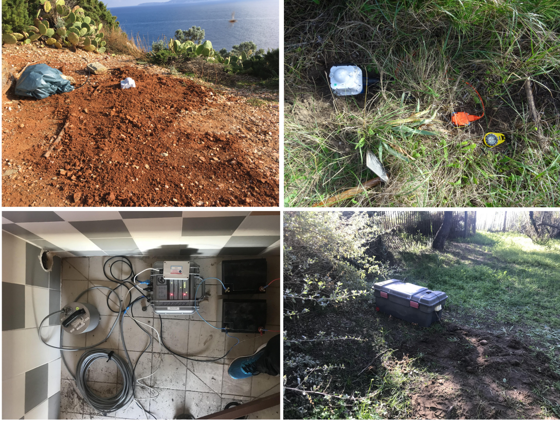
Figure 3: (Top row) Pictures of the installation of the MEMS accelerometers at the site PS05A (top left, Cap Bénat) and the site PS17 (top right, Almanarre beach). (Bottom row) Pictures of velocimeter installations in a building (bottom left) and in open field (bottom right).
