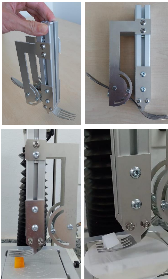
Figure 2. Actual images of the prototype, with a fork attached (up) and the system attached to a texturometer (down; Left: fork touching the carrot cube. Right: fork penetrating the starch gel).
