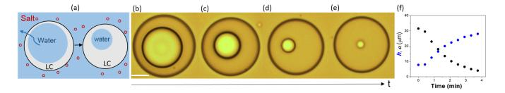
**Fig. 2** (a) Schematic illustration of the osmotic mechanism used to continuously vary the thickness of nematic shells (side view). (b)-(e) De-swelling process in a water/oil/water double emulsion when adding 10 wt%  $CaCl_2$  (top view). (f) During the process, the radius of the inner droplet a (black symbols) decreases, while the shell thickness h (blue symbols) increases. Scale bar: 25  $\mu$ m.
