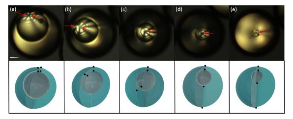
**Fig. 3** (a)-(e) Cross-polarized images of a shell (top view) with two pairs of +1 boojums at different stages of the de-swelling process. The red arrows indicate the location of the defects. The schematics below (side view) indicate the approximate position of the two pairs of +1 boojums (black dots) for each cross-polarized image. The time scale of the de-swelling process is of the order of 10 min. Scale bar:  $25 \mu m$ .
