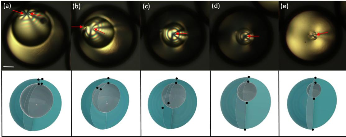
**Fig. 3** (a)-(e) Cross-polarized images of a shell (top view) with two pairs of +1 boojums at different stages of the de-swelling process. The red arrows indicate the location of the defects. The schematics below (side view) indicate the approximate position of the two pairs of +1 boojums (black dots) for each cross-polarized image. The time scale of the de-swelling process is of the order of 10 min. Scale bar:  $25 \mu\text{m}$ .
