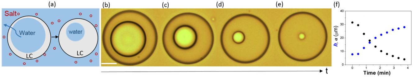
**Fig. 2** (a) Schematic illustration of the osmotic mechanism used to continuously vary the thickness of nematic shells (side view). (b)-(e) De-swelling process in a water/oil/water double emulsion when adding 10 wt%  $\text{CaCl}_2$  (top view). (f) During the process, the radius of the inner droplet  $a$  (black symbols) decreases, while the shell thickness  $h$  (blue symbols) increases. Scale bar:  $25 \mu\text{m}$ .
