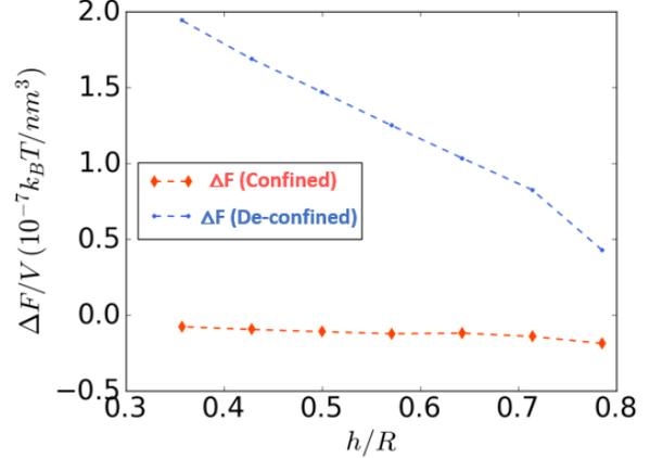
**Fig. 8** Energy barriers associated to the droplet expulsion for the confined and de-confined states as the inner droplet de-swells.
