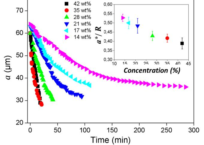
**Fig. 9** Variation of the inner droplet radius  $a$  as a function of time for different salt concentrations. Inset: critical inner radius  $a^*$  at which the droplet is expelled as a function of salt concentration.
