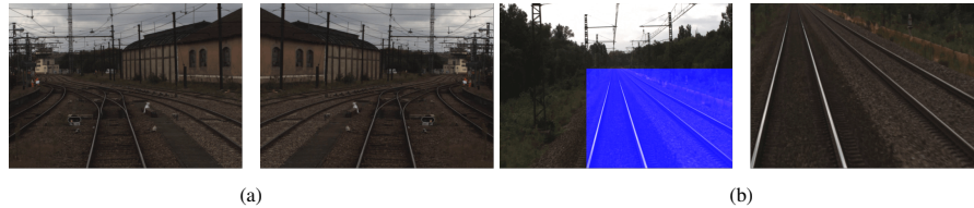
Fig. 3: Data augmentation. (a) Mirror via horizontal-shift augmentation, (b) Zooming to rails via image stretching transformation.
