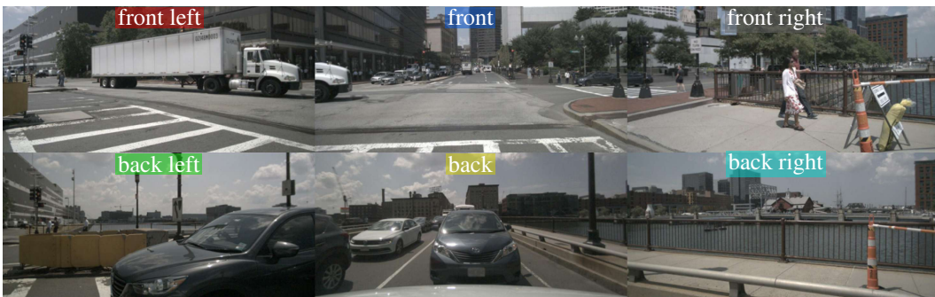
Figure 8: Six input camera images coming from the 360-degree camera rig of nuScenes. Note small overlaps between views, e.g., the front of the white truck is both seen in the front-left and front cams.
