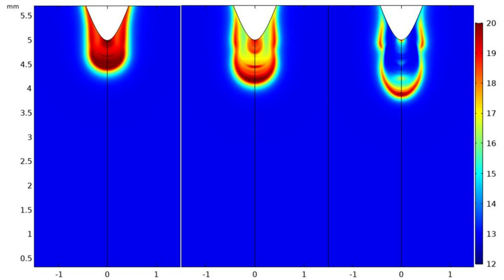
**Figure 8.** 2D surface plot of electron density profile at times 0.5, 1 and 2 ns in SF<sub>6</sub> at atmospheric pressure. Gap distance 5 mm,  $S_b = 10^{23} \text{ m}^{-3} \text{ s}^{-1}$ . Scaling parameter: 20 on logarithmic plot represents a density value of  $10^{20} \text{ m}^{-3}$ .
