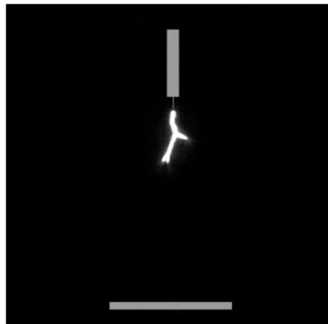
**Figure 11.** Photo (experiments) [31] of leader discharges in SF<sub>6</sub> at 1 bar in point to plane configuration. Needle radius of curvature = 0.2 mm, gap distance = 50 mm. Applied voltage = 107 kV.
