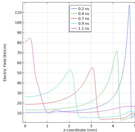
**Figure 18.** 1D line graph of the electric field for a streamer in SF<sub>6</sub> at 10 kPa when a voltage of 10 kV is applied.
