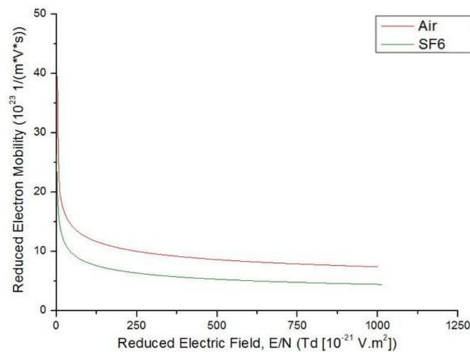
**Figure 2.** Reduced Electron Mobility as a function of Reduced Electric Field ( $E/N$ ) for  $\text{SF}_6$  [24] and air [26].
