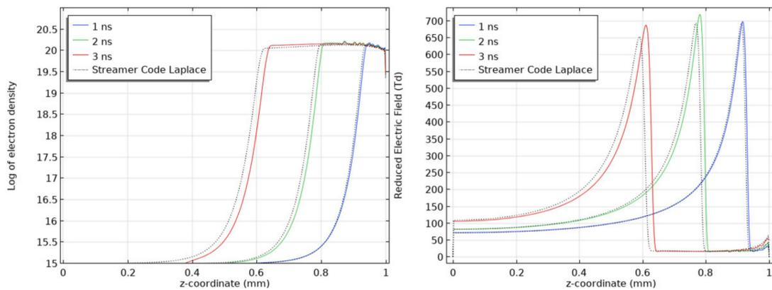
**Figure A2.** Electron density variation (left) and electric field distribution (right) on streamer axis at times  $t = 1, 2,$  and  $3$  ns for COMSOL™ model (solid line) and reference work by PRHE team, Laplace lab [33] (dotted line). No background ionization and no adaptive mesh used.
