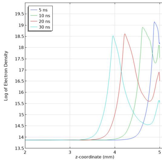
**Figure 19.** Line diagram along the symmetry axis of the log of the Electron Density profile for an applied voltage of 2 kV at pressure 10 kPa. Scaling parameter for density profiles: 20 on logarithmic plot represents a density value of  $10^{20} \text{ m}^{-3}$ .
