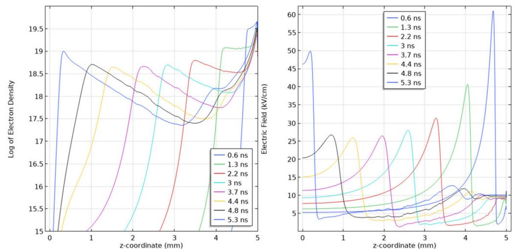
**Figure 14.** Line diagrams along the symmetry axis of the log of the Electron Density profile (left) and its corresponding Electric Field distribution (right) for a streamer propagating in a 5 mm SF<sub>6</sub> gap at a pressure of 10 kPa. Applied voltage of 5 kV. Scaling parameter for density profiles: 20 on logarithmic plot represents a density value of  $10^{20} \text{ m}^{-3}$ .
