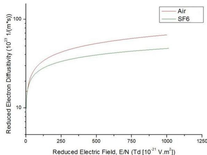
**Figure 3.** Reduced Electron Diffusivity as a function of Reduced Electric Field ( $E/N$ ) for  $\text{SF}_6$  [24,27] and air [25].
