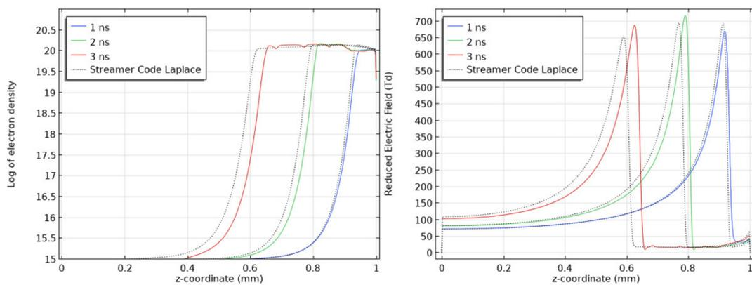
**Figure A3.** Electron density variation (left) and electric field distribution (right) on streamer axis at times  $t = 1, 2,$  and  $3$  ns for COMSOL™ model (solid line) and reference work by PRHE team, Laplace lab [33] (dotted line). Adaptive mesh used in COMSOL™ model.
