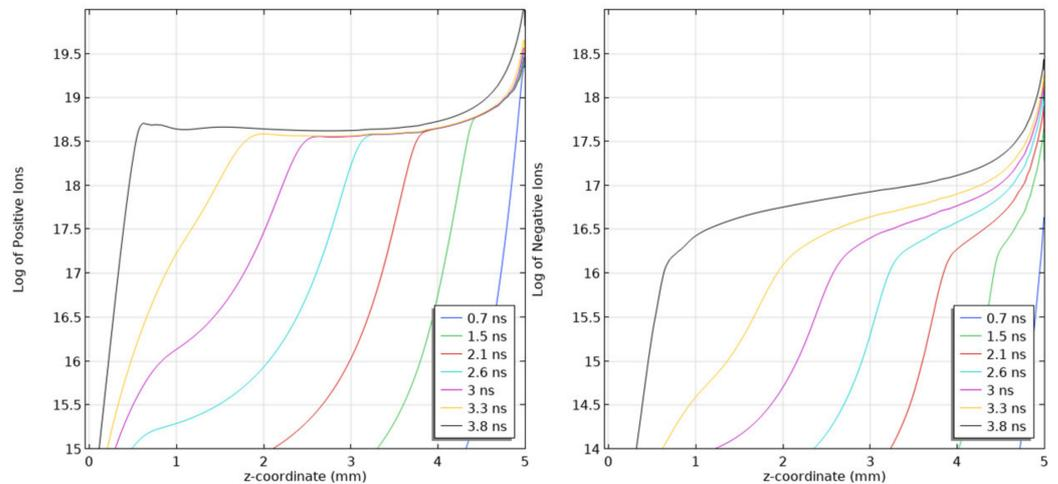
**Figure 13.** Line diagrams along the symmetry axis of the log of the Positive Ion Density profile (left) and the Negative Ion Density profile (right) for a streamer propagating in a 5 mm air gap at a pressure of 10 kPa. Applied voltage of 5 kV. Scaling parameter for density profiles: 20 on logarithmic plot represents a density value of  $10^{20} \text{ m}^{-3}$ .
