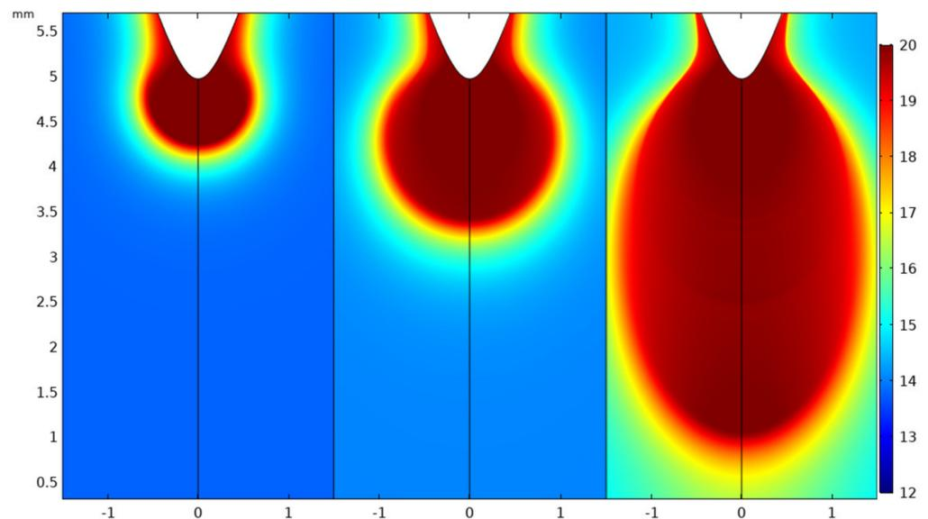
**Figure 5.** 2D surface plot of electron density profile at times 0.5, 1, and 2 ns in air at atmospheric pressure. Gap distance 5 mm,  $S_b = 10^{23} m^{-3} s^{-1}$ . Scaling parameter: 20 on logarithmic plot represents a density value of  $10^{20} m^{-3}$ .
