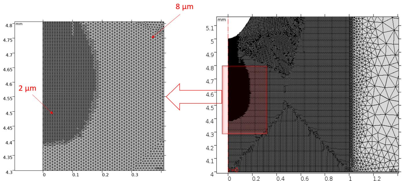
**Figure 4.** Mesh Sizes and Refinement.
