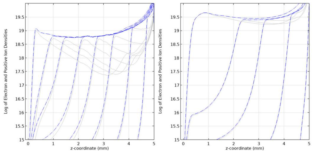
**Figure 17.** Line diagram of the positive ion density (blue dash-point lines) and electron density (solid gray lines) in SF<sub>6</sub> at 10 kPa when a voltage of 5 kV (**left**) and 10 kV (**right**) is applied. Scaling parameter for density profiles: 20 on logarithmic plot represents a density value of 10<sup>20</sup> m<sup>-3</sup>.
