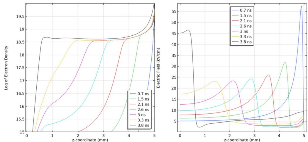
**Figure 12.** Line diagrams along the symmetry axis of the log of the Electron Density profile (**left**) and its corresponding Electric Field distribution (**right**) for a streamer propagating in a 5 mm air gap at a pressure of 10 kPa. Applied voltage of 5 kV. Scaling parameter for density profiles: 20 on logarithmic plot represents a density value of  $10^{20} \text{ m}^{-3}$ .
