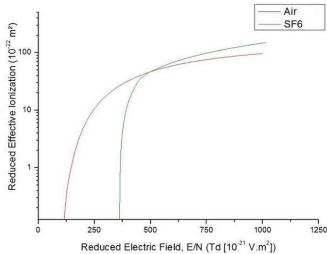
**Figure 1.** Reduced Effective Ionization as a function of Reduced Electric Field ( $E/N$ ) for  $\text{SF}_6$  [24] and air [25,26].
