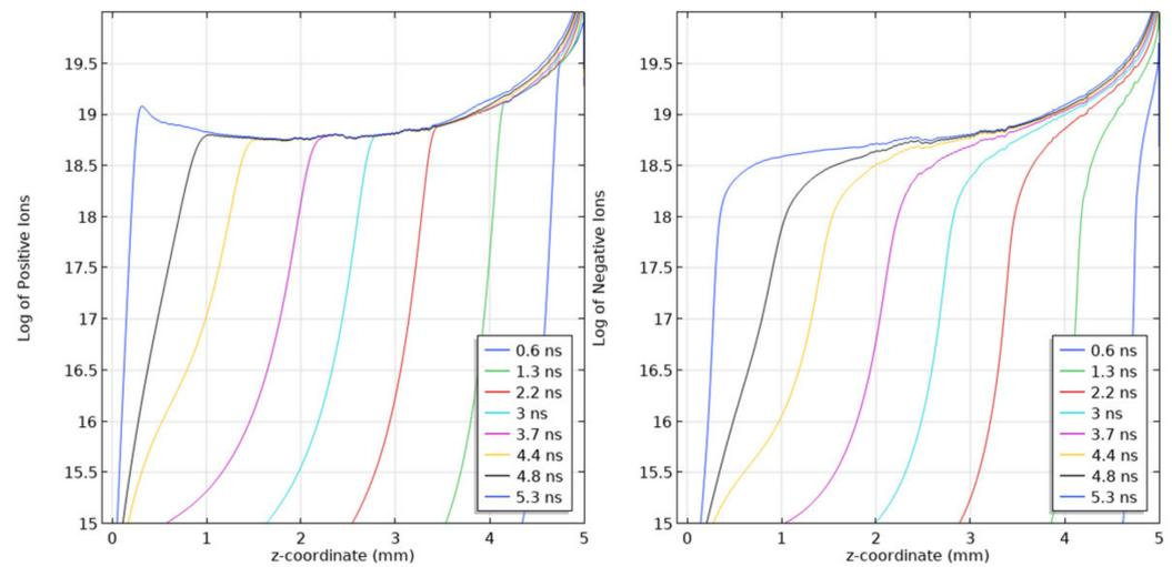
**Figure 15.** Line diagrams along the symmetry axis of the log of the Positive Ion Density profile (**left**) and the Negative Ion Density profile (**right**) for a streamer propagating in a 5 mm SF<sub>6</sub> gap at a pressure of 10 kPa. Applied voltage of 5 kV. Scaling parameter for density profiles: 20 on logarithmic plot represents a density value of  $10^{20} \text{ m}^{-3}$ .
