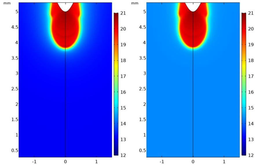
**Figure 10.** Surface plot of positive ion density profile (left) and negative ion density profile (right) at time 2 ns in SF<sub>6</sub> at atmospheric pressure. Scaling parameter: 20 on logarithmic plot represents a density value of 10<sup>20</sup> m<sup>-3</sup>.
