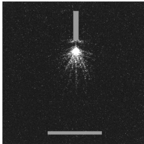
**Figure 16.** Photo (experiments) [31] of streamer discharges in SF<sub>6</sub> at 0.1 bar in point to plane configuration. Needle radius of curvature = 0.2 mm, gap distance = 50 mm. Applied voltage = 37 kV.
