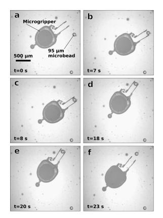
Fig. 7. In-liquid pick-and-place of a 95-µm diameter microbead using the proposed mobile microgripper. See the attached video.
