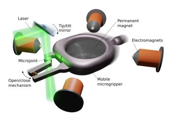
Fig. 1. Conceptual image of the proposed hybrid optothermalmagnetic mobile microgripper. The position of the microgripper is magnetically actuated and the gripping mechanism is optothermally actuated. The microgripper is approximately 1.5 mm in length.
