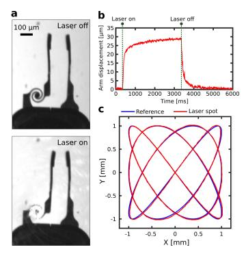
Fig. 5. Optothermal actuation of the microgripper showing its open and close states. (b) Step response of the gripping mechanism. (c) Performance of the laser steering system through a path following experiment of a Lissajous curve. The blue and red lines show the reference trajectory and the position of the laser spot, respectively.
