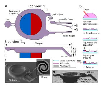
Fig. 2. Design and fabrication of the mobile microgripper. (a) Top view and side view of the proposed microgripper with its dimensions. (b) The full fabrication and release process of the microgripper. (c) SEM image of a fabricated microgripper before the release process. The inset shows a top view of the microjoint. (d) Image of a released microgripper with press fitted magnet.
