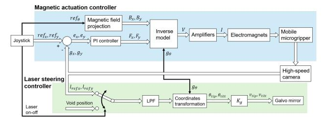
Fig. 4. Controller block diagram showing the magnetic actuation controller and the laser steering controller.
