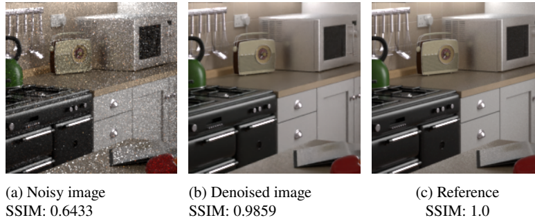
Fig. 9: Result of the U-Net Autoencoder denoising on one block of the Kitchen image with corresponding SSIM scores.
