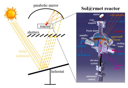
Fig. 13. Solar semi-continuous process for the regeneration of metal fuels through the carbo-thermal reduction of oxides. Adapted from [48].
