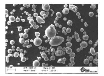
Fig. 9. Secondary-electron SEM image of the aluminum powder. Scale bar: 10  $\mu\text{m}.$
