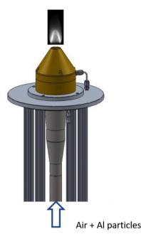
Fig. 8. Sketch of the Bunsen burner with the metal/air flame stabilized at the exit.
