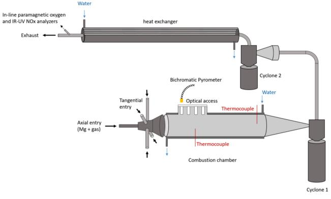
Fig. 5. Scheme of the magnesium-air burner. Adapted from [23].
