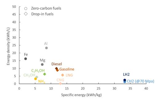
Fig. 2. Metal and efuels combustion enthalpies.
