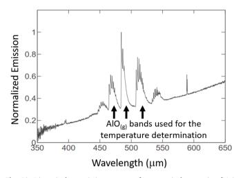
Fig. 12. Dimensionless emission spectrum for an equivalence ratio of 1.3, evidencing the vapor-phase nature of this combustion process.
