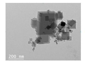
Fig. 7. TEM photographs of MgO particles (collected in the combustion chamber). Scale bar: 200 nm.
