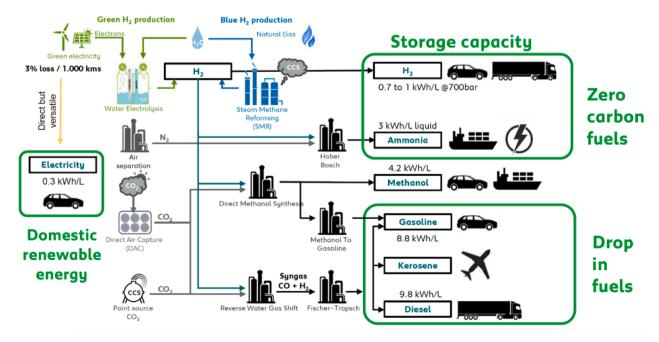
Fig. 1. Illustration of efuel production.
