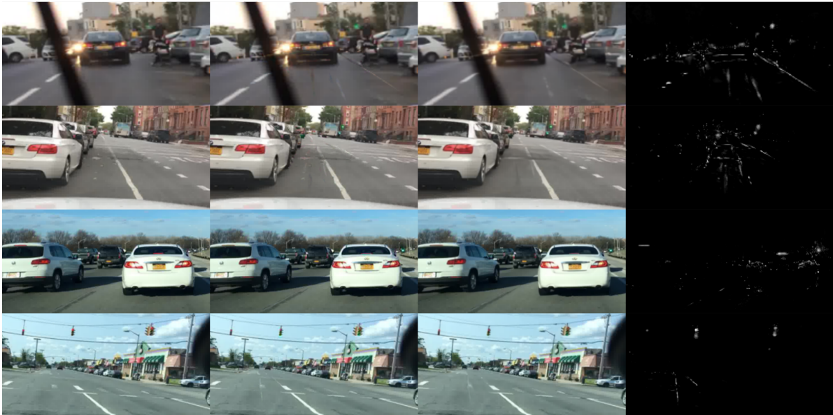
Figure 10. Additional BDD qualitative results. We show examples for the Forward / Slow Down binary class for \ell_1 distance loss. We show a zoom of the changes in the image since the perturbations are sparse. We see that ACE adds traffic light colors in the buildings to change the prediction.
