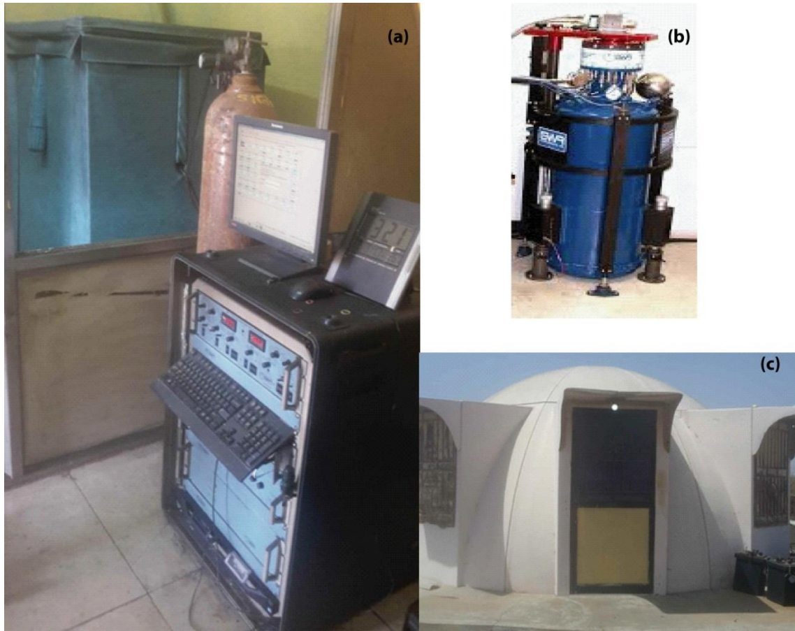
113 Figure 2: Superconducting Gravimeter placed in Badargadh station, Gujarat, India, a) DAC unit, 114 b) Dewar and c) the dome structure
