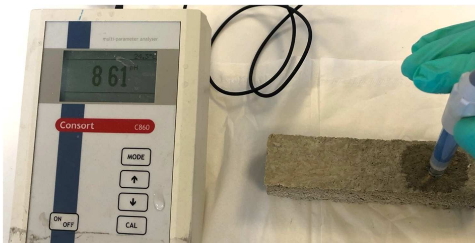
Figure 8. Measurement of the surface pH level using a WTW Sentix Sur electrode
