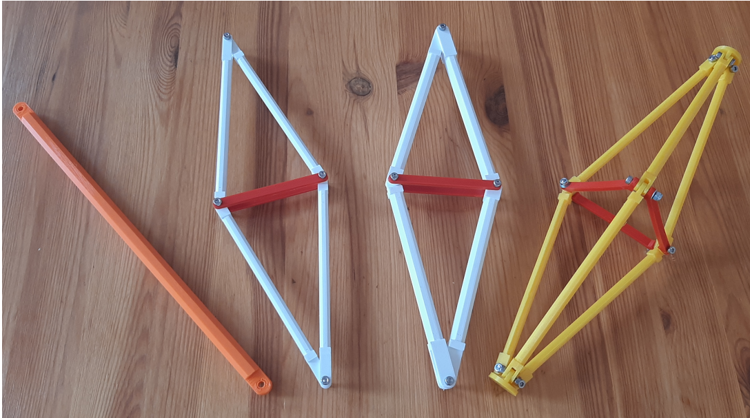
Figure 5: 3D printed braces: (a) Straight column; (b) light 2D D-bar; (c) heavy 2D D-bar; (d) 3D D-bar.
