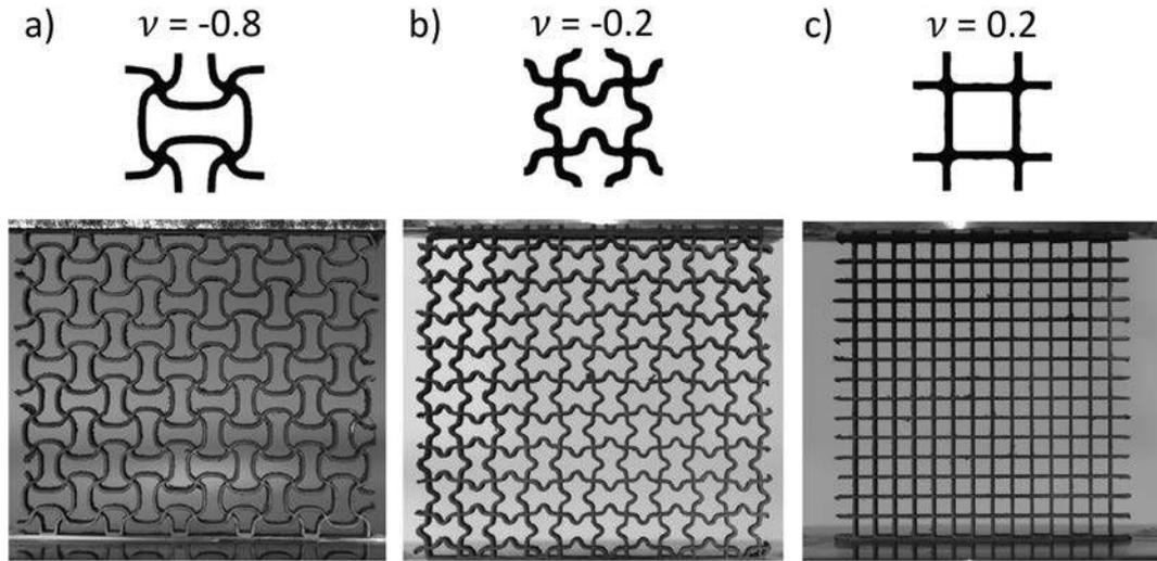
**Fig. 1.** Pictures of the 3 specimens manufactured by Directed Energy Deposition and tested under a compression load. Their design is originally based on an auxetic cell extracted from (Clausen et al., 2015) with a Poisson ratio of  $-0.8$ ,  $-0.2$  and  $0.2$  in a), b) and c) respectively. The geometric details of the 3 fabricated specimens are available in Table 1.
