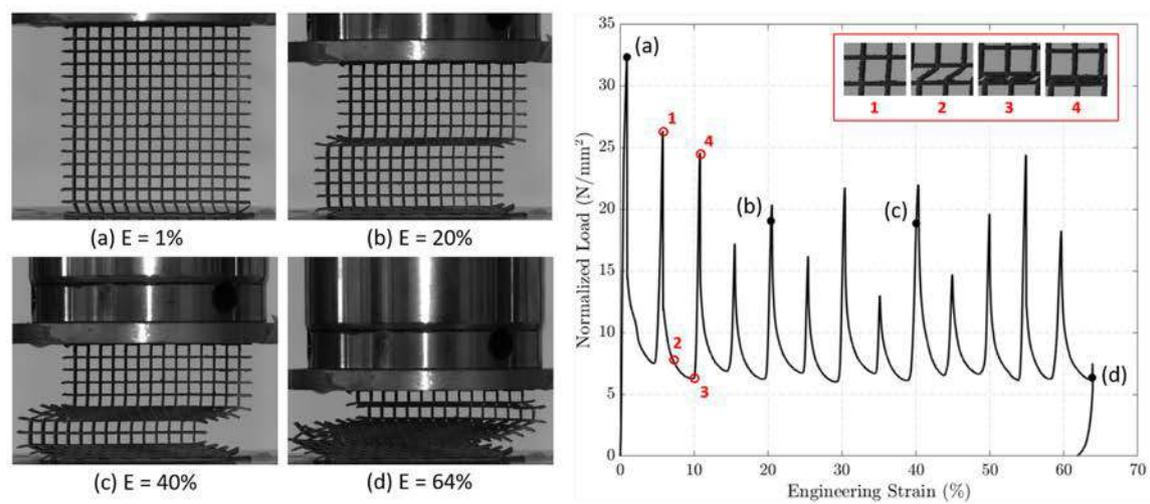
**Fig. 4.** Experimental compression test results. Snapshots taken for various engineering strain levels. Measured load normalized by the specimen section versus engineering strain.
