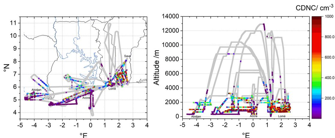
**Figure 2.** Flight paths of the DLR Falcon research aircraft during the DACCIWA airborne measuring campaign from 29 June until 14 July 2016. Based in Lomé, Togo, 12 research flights in total led across the West African neighboring countries of Côte d'Ivoire, Ghana and Benin, as well as of segments above the Gulf of Guinea. Measured cloud sequences from the CAS-DPOL are color-coded along the flight tracks.
