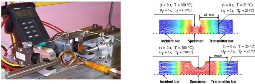
**Fig. 1.** a) Hot SHPB rapid compression test device, b) Comparisons of Finite Element temperature fields obtained after a time of 5s corresponding to a material cooling from a setting temperature of  $500^\circ\text{C}$  reached by a rapid induction heating in the case of an uniform cylindrical specimen and of a dumbbell shape sample [1].
