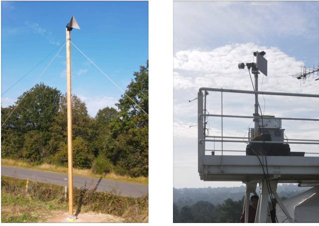
(a) Corner reflector (at 8 m height) (b) Radar antenna (at 15 m height) Fig. 3. Calibration measurement set-up
