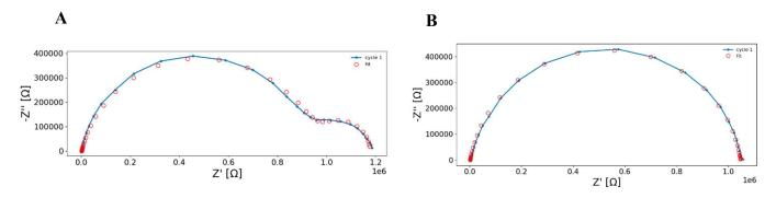
Figure 3: EIS plot on the same microfluidic channel with 3 mM of ferri/ferrocyanide diluted in 0.5 NaCl, for different flow rate:  $0.01 \,\mu\text{L/s}$  (A) and  $1 \,\mu\text{L/s}$  (B).
