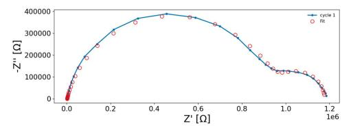
Figure 2: Example of experimental data and its corresponding fitting procedure. This example is referring to an experiment performed with Q=0.01 μL/s, the minimum working flow that can be set using the model of neMESYS syringe pump available. (A) Nyquist EIS plot, experimental data (blue curve) and fitting model (red circle).
