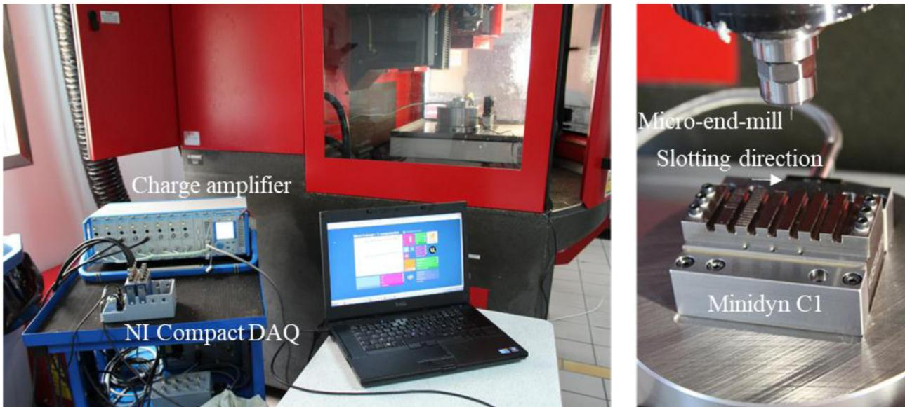
**Fig. 7.** The experimental configuration for the micro-milling tests.
