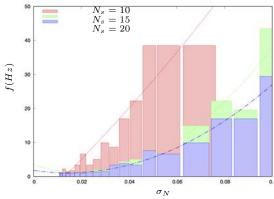
Fig. 5: Frequency sampling f providing a 95% success for source identification versus r.m.s noise  $\sigma_N$  for randomly generated graphs having maximum vertex degree  $\Delta(G)=3$ , minimum vertex degree  $\delta(G)=2$ , N=100 nodes and randomly chosen sources.Dotted lines are quadratic fit of the results to help delineate the upper region for which the  $f-\sigma_{SN}$  values offer a 95% confidence for source detection.
