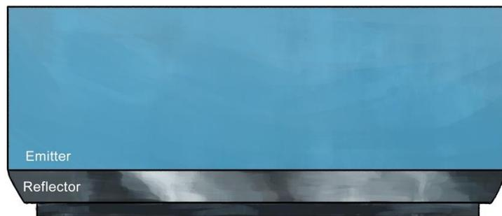
Figure 2 - Sketch of the simple two-layer coating
