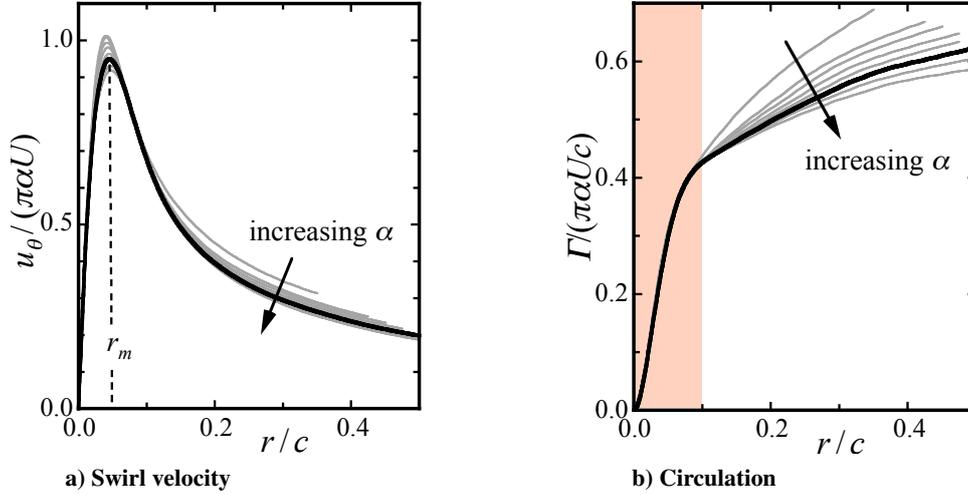
**Fig. 5.** Radial velocity and circulation profiles (azimuthal averages) of the tip vortex at  $x/c = 6$ , for  $\alpha$  in the range  $4^\circ$ – $12^\circ$ . The thick lines show the results for  $\alpha = 10^\circ$ .
