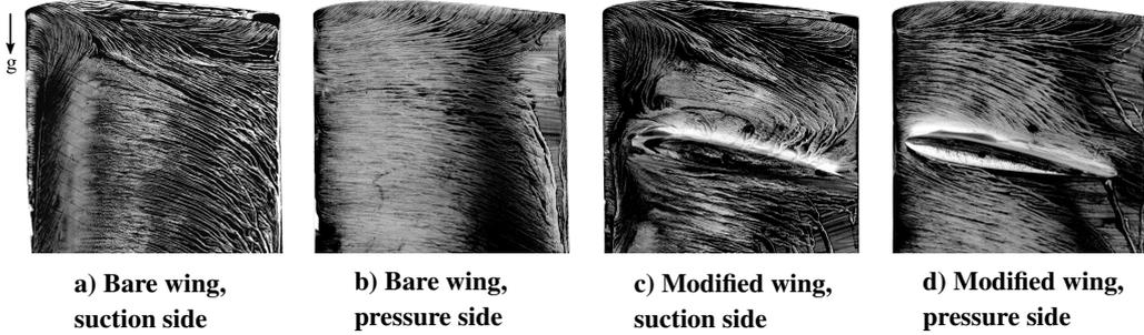
**Fig. 6.** Oil flow pattern for the reference case and a modified configuration at  $Re = 100,000$  and  $\alpha = 10^\circ$ . For a better comparison, the pressure sides are mirrored. Fin geometry for (c,d):  $d/c = 0.5$ ,  $h/c = 0.3$ ,  $\alpha_f = 10^\circ$ , flow is from left to right.
