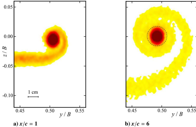
**Fig. 4.** Streamwise vorticity distribution at two downstream positions behind the bare wing at  $\alpha = 10^\circ$ . The dashed circle in (b) has a diameter of  $0.2c$ .
