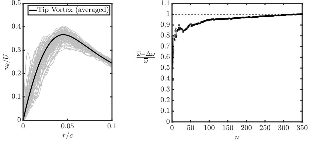
**Fig. 3.** (a) Instantaneous swirl velocity profiles of the tip vortex; the black line represents the profile obtained from the averaged velocity field. (b) Convergence ratio of the streamwise vorticity component  $\omega$  at a point within the tip vortex core.
