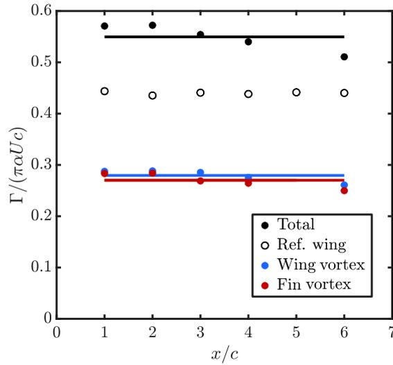
**Fig. 13.** Vortex circulations in the co-rotating system.
