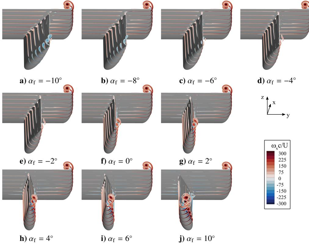
**Fig. 9.** Vortex formation at the fin and wingtips for different fin angles, illustrating the effect of the cross flow close to the wingtip. The neutral position (no fin vortex) is shifted to  $\alpha_f \approx -5^\circ$ .  $d/c = 0.3$  and  $h/c = 0.3$  for all cases.
