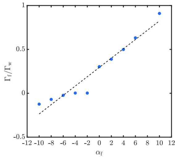
**Fig. 22.** Circulation ratio immediately behind the wing trailing edge as function of the fin angle. Data obtained from numerical simulations for  $\alpha = 10^\circ$ ,  $d/c = 0.3$  and  $h/c = 0.3$  (see also Fig. 9).
