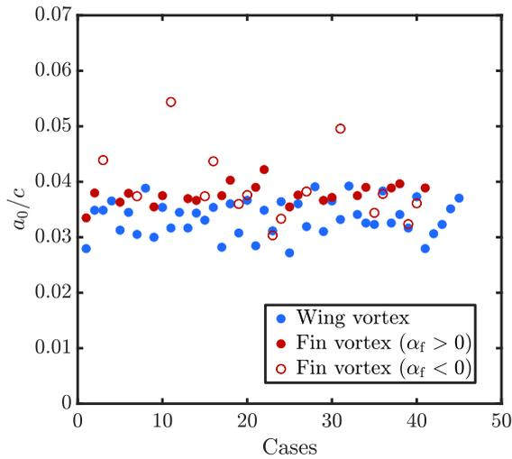
**Fig. 18.** Gaussian core radius  $a$  for all configurations.
