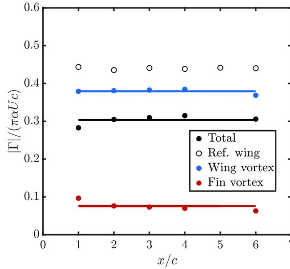
Fig. 15. Vortex circulations in the counter-rotating system.
