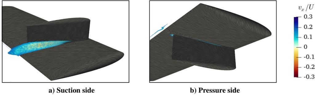
**Fig. 8.** Illustration of the separation tendency close to the fin root **at an angle of attack of  $\alpha = 10^\circ$**  for a fin position on (a) the suction and (b) the pressure side of the main wing. Fin geometry:  $d/c = 0.5$ ,  $h/c = 0.3$ ,  $\alpha_f = 10^\circ$ .
