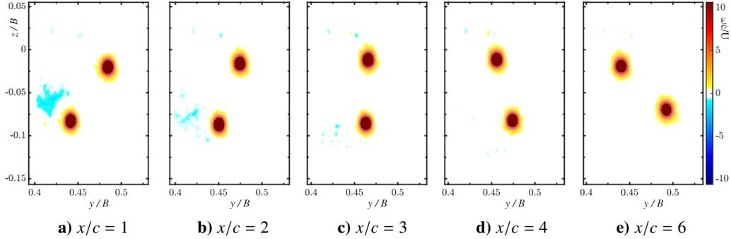
**Fig. 10.** Vorticity fields in different planes behind the wing, illustrating the development of a co-rotating vortex system. The fin parameters are:  $d/c = 0.3$ ,  $h/c = 0.3$ ,  $\alpha_f = 10^\circ$ .
