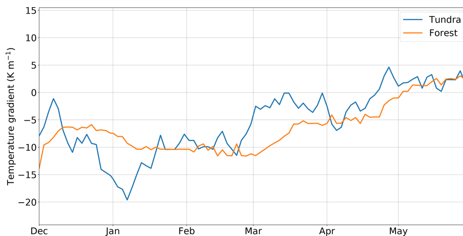
Figure 11. Temperature gradient at the base of the snowpack for winter 2017–2018 at TUNDRA and FOREST. At TUNDRA, measurements were made at 11 and 21 cm, while the measurement heights were 4 and 14 cm at FOREST. Note that the measurement interval was 2 d; thus the peak gradients are likely to be larger than shown here. Negative gradients indicate higher temperatures close to the ground surface than those in higher snow layers.
