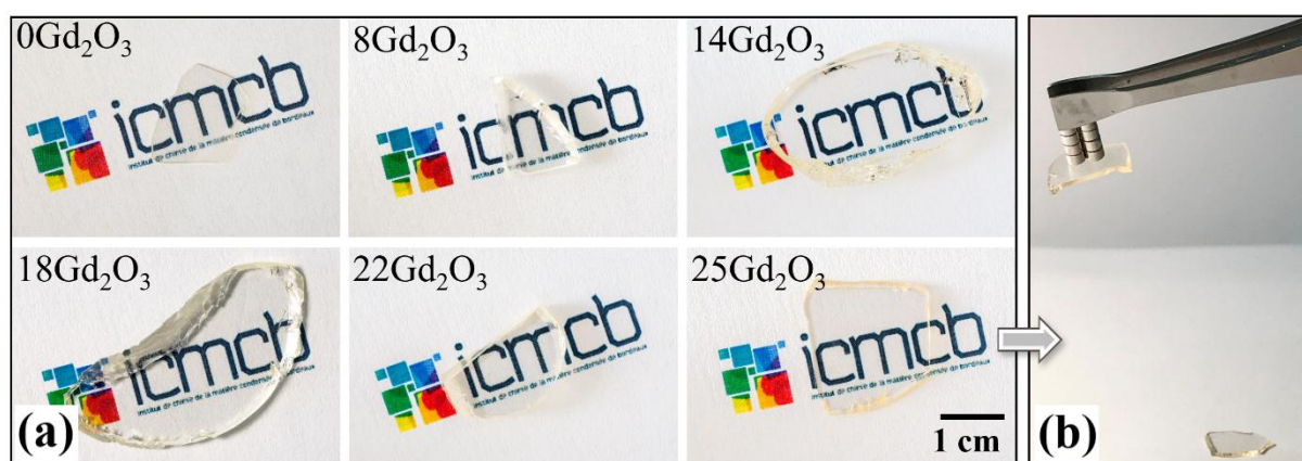
Fig. 1. a) A photograph of glasses from 0 up to 25 mol% of \text{Gd}_2\text{O}_3 after cutting and polishing; b) sample with 25 mol% of \text{Gd}_2\text{O}_3 attracted by the magnet.
