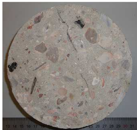
Figure 10 Surface of 0S-100G concrete after heating–cooling up to 300 °C
