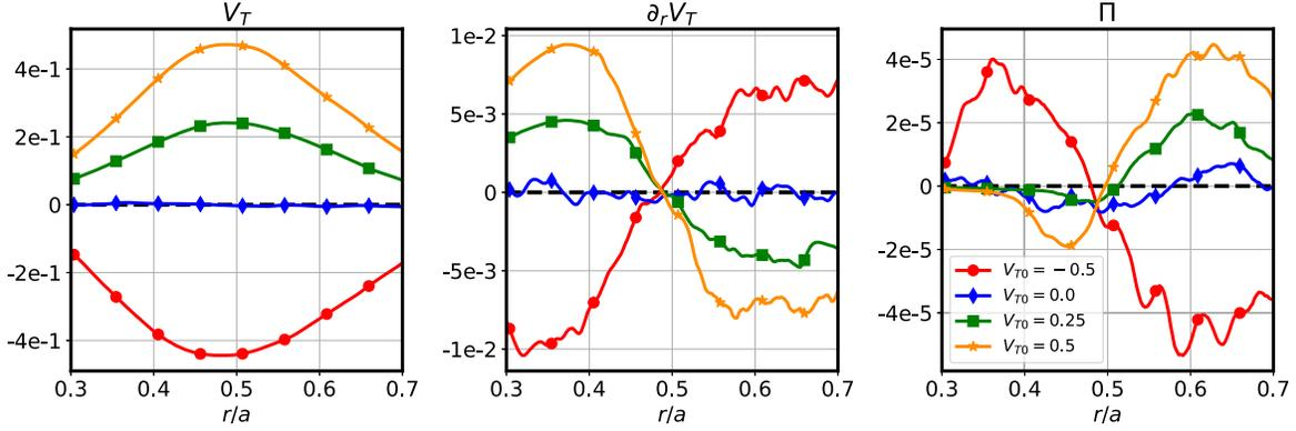
FIG. 2. Radial profiles of the toroidal velocity  $V_T$ , its shear  $V_T'$ , and the stress tensor  $\Pi$  taken at turbulent saturation for simulations without ripple and with different initial toroidal velocity profiles  $V_T(t=0) = V_{T0} \exp[-32(r/a - 0.5)^2]$  with  $a$  the minor radius. Velocities are normalized to the ion thermal velocity and lengths to ion Larmor radius  $\rho_i$ .
