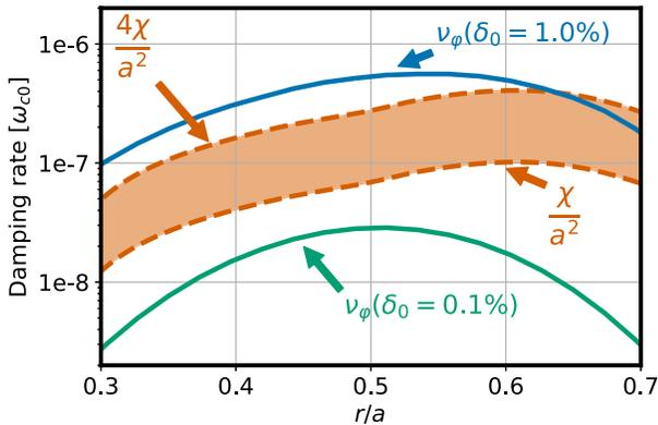
FIG. 3. Radial profile of magnetic drag  $\nu_\phi$  for different ripple amplitudes and the turbulent viscous contribution  $\chi\lambda_v$ . Orange zone represents  $\chi|\lambda_v|$  for  $a/2 \leq |\lambda_v|^{-1/2} \leq a$ . Time is normalized to the cyclotron period  $\omega_{c0}^{-1}$ .
