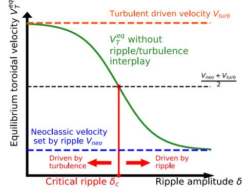
FIG. 1. Sketch of the modeled ripple-turbulence competition on the equilibrium toroidal velocity estimated with local momentum conservation in the case of cocurrent  $V_{\text{turb}}$ . The synergistic effects are not accounted for here, but are detailed further below.
