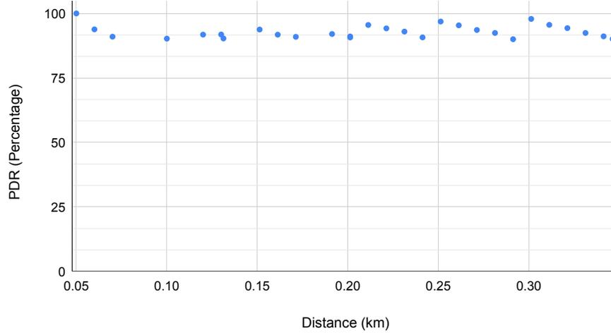
Fig. 9: Low load (density  $\rho$  of 90 nodes per  $\text{km}^2$ , traffic intensity of  $1/12.33 \text{ min}^{-1}$ ), SF boundaries for target PDR of 90%, Rayleigh fading. Cell capacity around 30 nodes.
