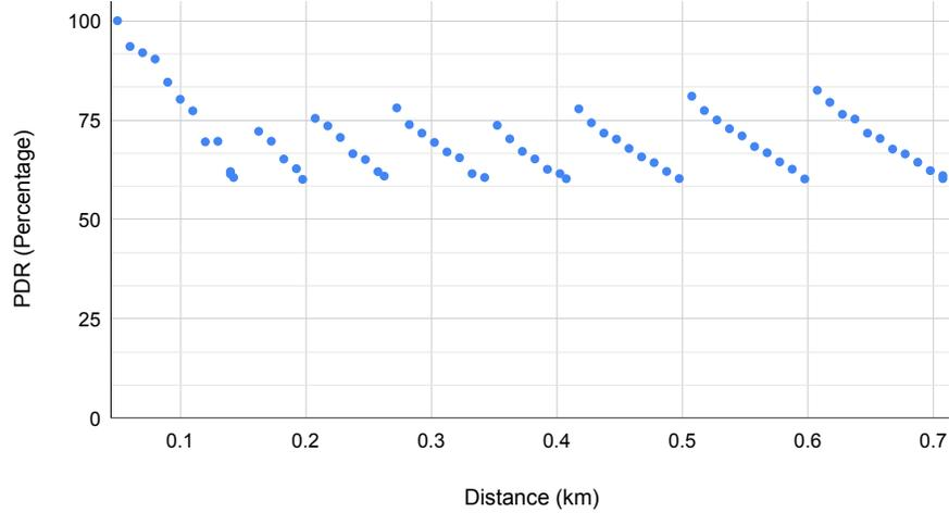
Fig. 8: Low load (density  $\rho$  of 90 nodes per  $\text{km}^2$ , traffic intensity of  $1/12.33 \text{ min}^{-1}$ ), SF boundaries for target PDR of 60%, Rayleigh fading. Cell capacity around 140 nodes.
