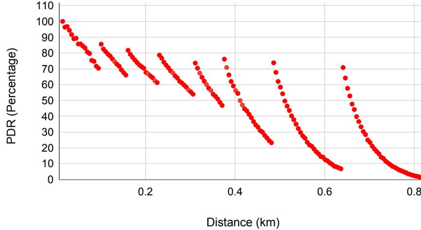
Fig. 3: Case of SNR boundaries and maximal load in the standard LoRa: cell radius of 0.636 km, node density  $\rho$  of 900 nodes per  $\text{km}^2$ , Rayleigh fading. Around 220 nodes in the distance of 0.280 km from gateway, using up to SF8 receive a PDR of at least 60%. Traffic intensity limited by the 1% duty cycle in the standard LoRa ( $1/12.33 \text{ min}^{-1}$ ).
