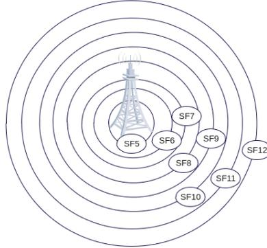
Fig. 1: Annuli of SF allocation around the gateway (the SF boundaries are equidistant in the figure, which is not the case in reality).
