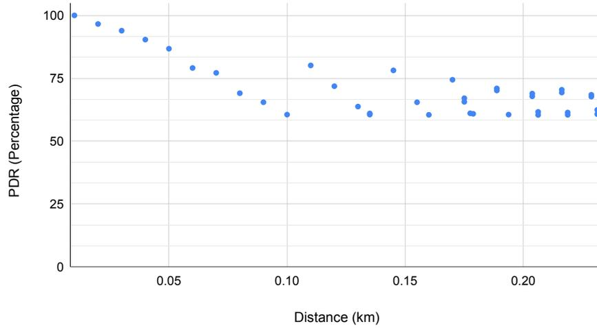
Fig. 10: High load (density  $\rho$  of 900 nodes per  $\text{km}^2$ , traffic intensity of  $1/2 \text{ min}^{-1}$ ), SF boundaries for target PDR of 60%, Rayleigh fading. Cell capacity around 150 nodes.
