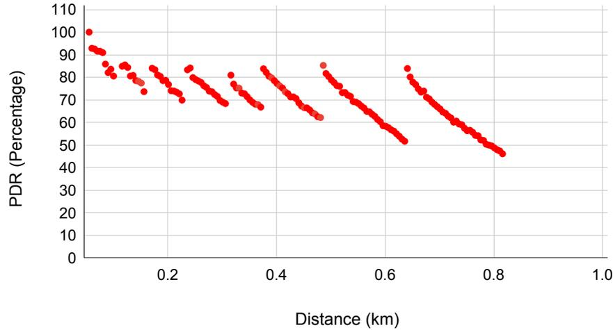
Fig. 2: Case of SNR boundaries and maximal load in the standard LoRa: cell radius of 0.636 km, node density  $\rho$  of 90 nodes per  $\text{km}^2$ , Rayleigh fading. Around 100 nodes in the distance of 0.590 km from gateway, using up to SF11 receive a PDR of at least 60%. Traffic intensity limited by the 1% duty cycle in the standard LoRa ( $1/12.33 \text{ min}^{-1}$ ).
