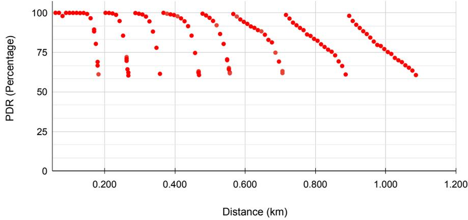
Fig. 4: Low load (density  $\rho$  of 90 nodes per  $\text{km}^2$ , traffic intensity of  $1/12.33 \text{ min}^{-1}$ ), SF boundaries for target PDR of 60%, Rician fading. Cell capacity around 310 nodes.
