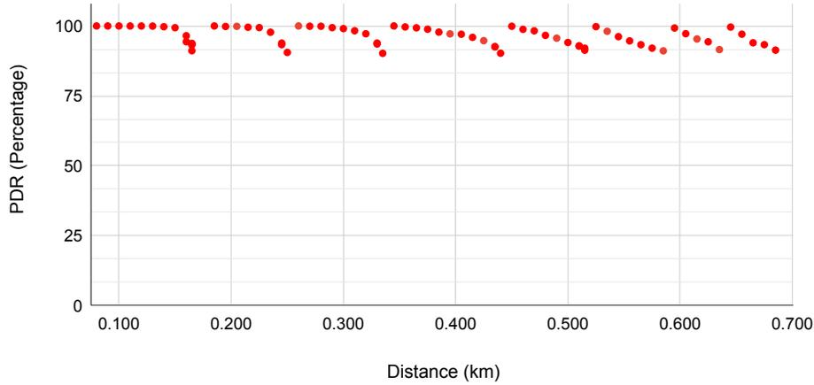
Fig. 5: Low load (density  $\rho$  of 90 nodes per  $\text{km}^2$ , traffic intensity of  $1/12.33 \text{ min}^{-1}$ ), SF boundaries for target PDR of 90%, Rician fading. Cell capacity around 120 nodes.
