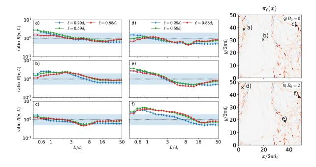
FIG. 7. Ratio  $R(\boldsymbol{x},L) = -\langle \pi_\ell \rangle / \langle \boldsymbol{u} \cdot \boldsymbol{d}_\nu + \boldsymbol{b} \cdot \boldsymbol{d}_\eta \rangle$  between the local cascade rate and the local dissipation rate averaged on a cubic region of size L centered around a given point  $\boldsymbol{x}$ . The results for three different points on the plane  $z = 25 \times 2\pi d_i$  in run I (a-c) and run II (d-f) are shown. The shaded region individuates the interval 0.5 < R < 2.
