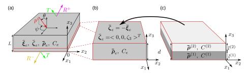
Figure 1: [Color online] Sketch of a *L*-thich layer of a general Willis fluid (a), of the *d*-thick unit cell of the Willis fluid, and of the two-orthotropic fluid laminate unit cell (c).
