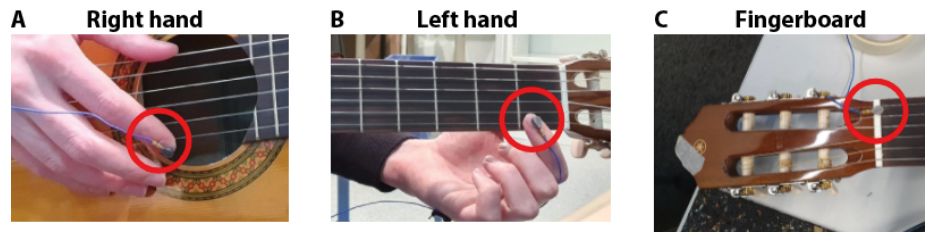
Fig. 1. Measurement of the string’s vibration with an accelerometer placed at several locations. A) On the right hand’s index finger. B) On the left hand’s index finger. C) On the guitar fingerboard
