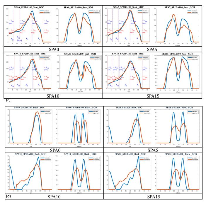
Figure 6. Comparison of simulated pressure distribution and profiles with experimental data for the four seat pan angles (SPA: 0°, 5°, 10° and 15°). (a) pressure on the seat pan, (b) pressure on the backrest, (c) lateral (SOC) and frontal (SOR) pressure profiles on the seat pan, (d) lateral (SOC) and frontal (SOR) pressure profiles on the backrest.
