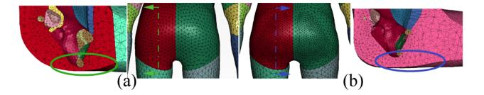
Figure 3 Local refinement of the soft tissue mesh under the ITs (a) mesh of the child model(b) refinement of the local mesh of buttocks with the adult model.
