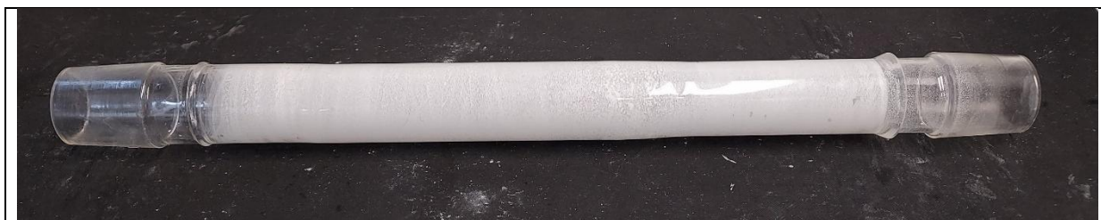
Fig.S1: Tubular Pyrex reactor coated with 200 mg of photocatalyst
