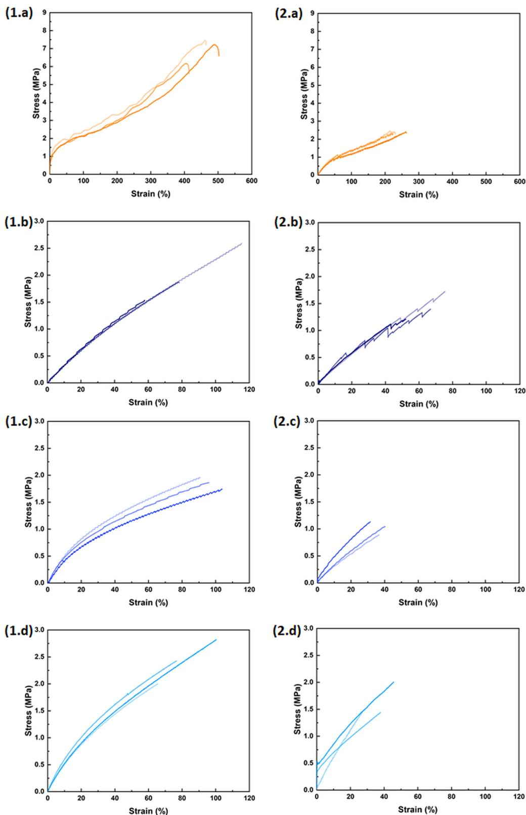
**Figure 4.** Mechanical evaluation of the networks by tensile tests. Stress–strain curves in the (1) dry state at room temperature and in the (2) hydrated state at 37 °C of (a) PEG<sub>10k</sub>-PLA<sub>40k</sub>, (b) PEG<sub>20k</sub>-PLA<sub>7.5k</sub>, (c) PEG<sub>20k</sub>-PLLA<sub>7.5k</sub>, and (d) PEG<sub>20k</sub>-PLLA<sub>7.5k</sub>/PEG<sub>20k</sub>-PDLA<sub>7.5k</sub>.
