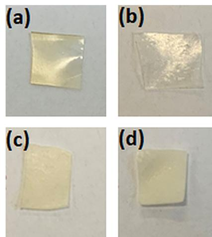
**Figure 2.** Visual aspect of the networks. Pictures of the different materials after crosslinking: (a) PEG<sub>10k</sub>-PLA<sub>40k</sub>, (b) PEG<sub>20k</sub>-PLA<sub>7.5k</sub>, (c) PEG<sub>20k</sub>-PLLA<sub>7.5k</sub>, and (d) PEG<sub>20k</sub>-PLLA<sub>7.5k</sub>/PEG<sub>20k</sub>-PDLA<sub>7.5k</sub>.
