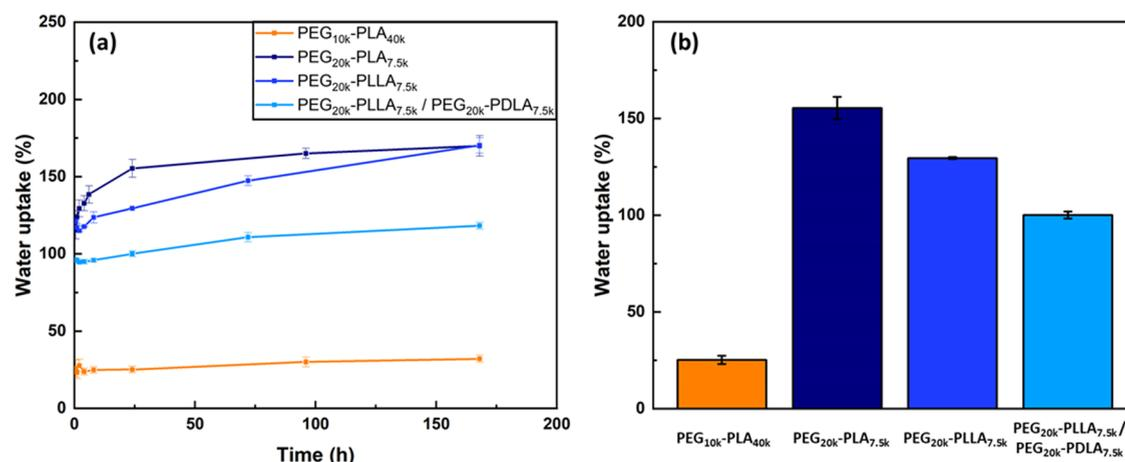
**Figure 3.** Water uptake of the networks. (a) Evolution of water uptake in PBS with time. (b) Water uptake after 24 h in PBS. Data are expressed as the mean  $\pm$  SD and correspond to measurements with  $n = 3$ .
