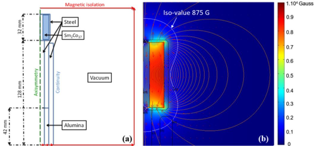
**FIG. 4.** (a) Schematic of the dipolar ECR source showing different magnetic domains and the boundary conditions used in the “Magnetostatics” module. (b) Mapping of magnetic flux density, magnetic field lines, and iso-value line at 875 G for a single dipolar magnet source. The top and the bottom of the magnet are set to North and South pole, respectively.
