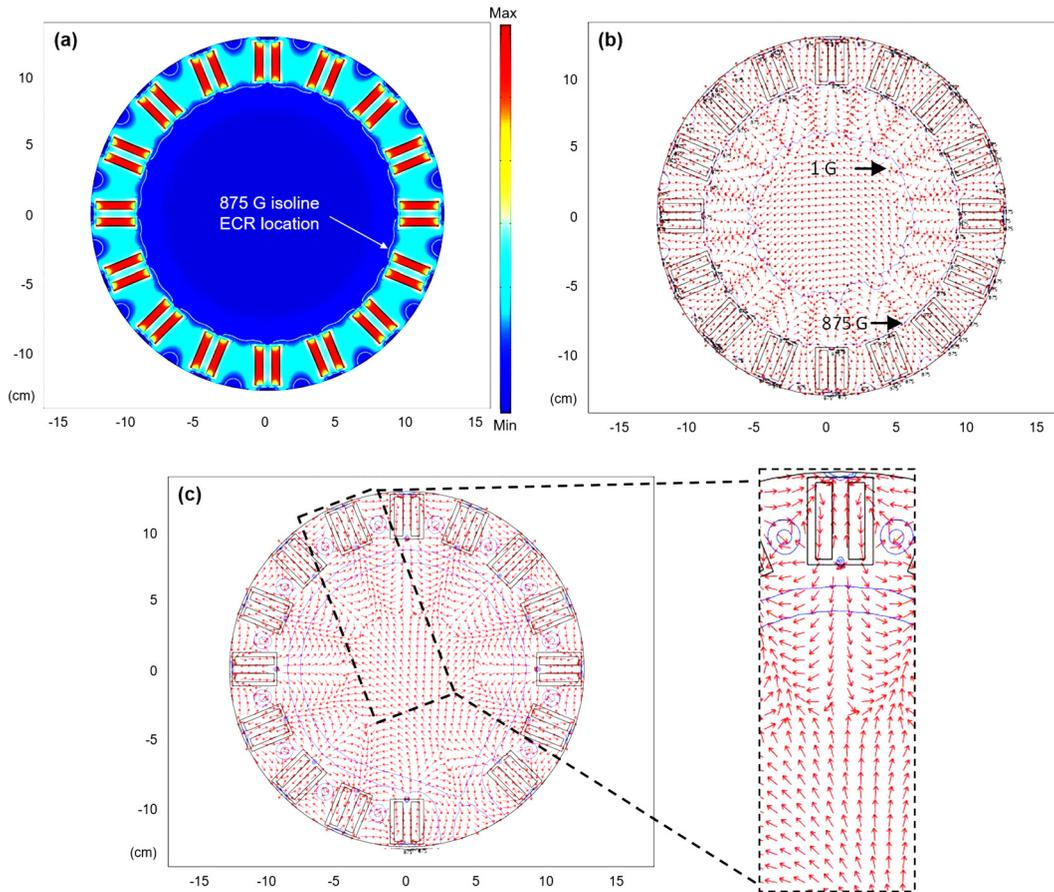
**FIG. 7.** (a) Mapping of the magnetic flux density, (b) field lines and iso-value lines created by 16 ECR sources with alternating polarity, and (c) field lines and iso-value lines created by 15 ECR sources with alternating polarity.
