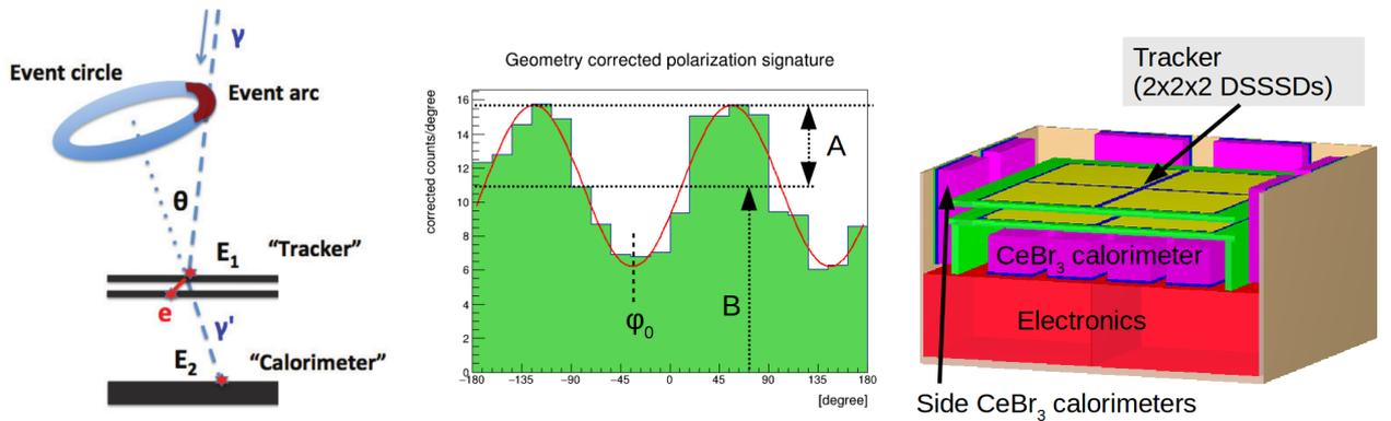
**Fig. 1. Left:** Scheme of a Compton telescope. **Middle:** Polarization signature (cosine squared modulation) in a Compton telescope (from simulations). The angle of polarization is  $\phi_0$  and the fraction of polarization is  $\frac{A/B}{\mu_{100}}$ , where  $\mu_{100}$  is the amplitude of the modulation of a 100% polarized source. **Right:** 4U scientific payload of COMCUBE (6U).
