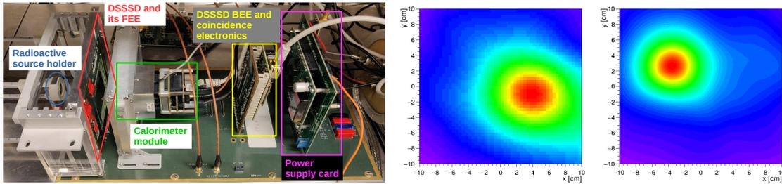
**Fig. 4. Left:** Picture of the first prototype with its main components. FEE and BEE stand respectively for Front-End Electronics (analog signal processing and digitization) and Back-End Electronics (data merging and communication with onboard computer) **Right:** Reconstructed images for two positions of the  $^{137}\text{Cs}$  source. Source positions were  $x, y = (36, -11) \text{ mm}$  and  $x, y = (-36, 23) \text{ mm}$ .
