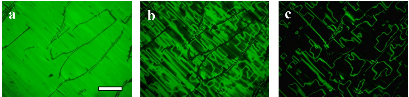
Figure 11. SmA b sample at T = 88.0 °C under electric field: a) U = 3.09 V rms ; b) U = 4.24 V rms ; c) U = 4.80 V rms ( f = 6 kHz). The cell is observed under a polarizing microscope with a Senarmont
