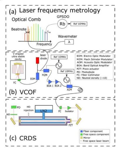
FIG. 1. Experimental set-up developed in Grenoble. The figure is structured in three blocks, detailing from top to bottom, (a) the frequency calibration, (b) the light source and (c) cavity ring-down spectrometer, respectively. GPSDO stands for GPS Disciplined Oscillator, VCOF stands for V-shaped Cavity-Based Optical Feedback and LN2 for liquid nitrogen. The Acousto-Optic Modulator AOM is driven at 88.5 MHz.
