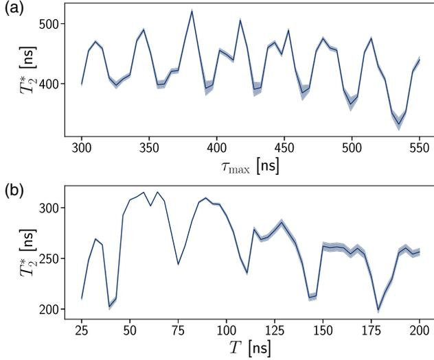
FIG. 14. Feedback performance for a single-species unitary algorithm. (a),(b) Simulated  $T_2^*$  versus maximum sensing time  $\tau_{\max}$  and actuation time  $T$ , respectively. The evolution during the feedback algorithm is entirely unitary, except for the explicit dissipative reset step. Here we use the model parameters found in Appendix E 6, but we only simulate a single nuclear species with Zeeman frequency  $\omega_n = 29$  MHz. Shaded regions represent the 68% confidence intervals.
