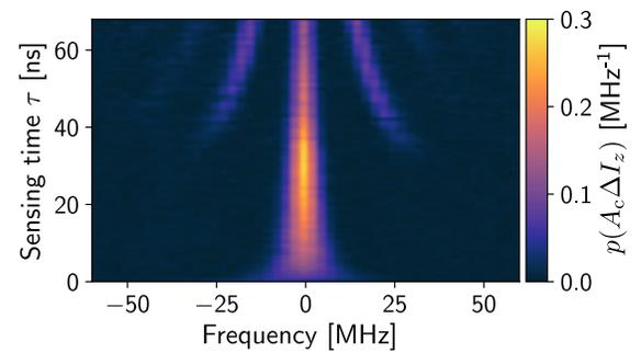
FIG. 9. Minimum capture range. 2D plot of  $p(A_c \Delta I_z)$  versus frequency,  $A_c \Delta I_z$ , and sensing time  $\tau$ . In this experiment we do not dynamically sweep the sensing time, but rather use a constant value for all 44 repeats (per preparation cycle) of the algorithm. For sufficiently small  $\tau \lesssim 35$  ns we avoid multistability and prepare a single-mode distribution.
