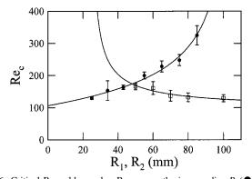
FIG. 6. Critical Reynolds number  $Re_c$  versus the inner radius  $R_1(\bullet)$  (the outer radius being constant  $R_2 = 105$  mm), and versus the outer radius ( $\square$ ) (the inner radius being constant  $R_1 = 25$  mm). Here h = 5 mm. The continuous lines correspond in each case to  $Re = 100 C^{-1/2}$ .
