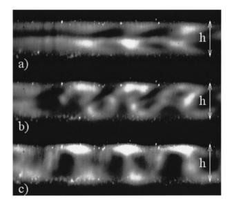
FIG. 4. Evolution of the flow structure in the thickness of the cell, observed at  $\theta$ =135° from upstream at increasing flow rates: (a) Re=183, (b) Re=227, and (c) Re=277 (h=5 mm,  $R_1$ =25 mm, and  $R_2$ =105 mm). The image shows a part of the radial extension of the cell: The right edge corresponds to r=40 mm and the left edge to r=80 mm. Figure 4(c) looks unfocused as it is a time average of nonstationary structures.
