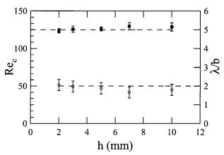
FIG. 5. Evolution with the cell thickness h of the critical Reynolds number  $\text{Re}_c$  (left and  $\blacksquare$ ) and the dimensionless wavelength  $\lambda/h$  (right and  $\bigcirc$ ). Here  $R_1 = 25 \text{ mm}$  and  $R_2 = 105 \text{ mm}$ .
