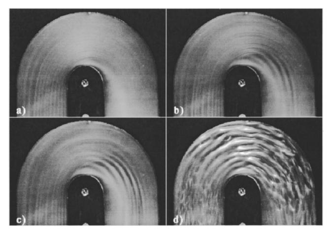
FIG. 3. Different patterns observed from above (for h=5 mm,  $R_1=25$  mm, and  $R_2=105$  mm) at increasing flow rates: (a) Re=62, (b) Re=130, (c) Re=172, and (d) Re=340. The flow is clockwise. Note that some streaks are visible at the bottom left of each figure; they are not related to any instability but to structures created by straws at inlet. These structures are damped but remain visible as fossil streaks.
