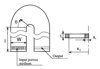
FIG. 1. Experimental set-up. l=20 cm,  $W=R_1-R_2$  and h,  $R_1$ , and  $R_2$  have been varied in the range: 2 < h < 10 mm,  $25 < R_1 < 75$  mm, and  $40 < R_2 < 105$  mm.
