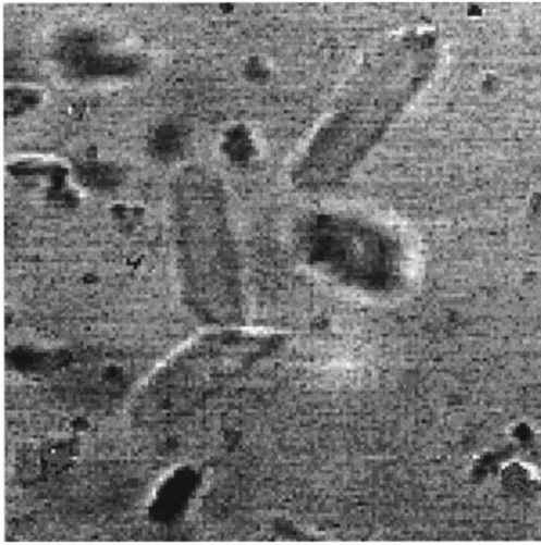
FIG. 4. Photograph under microscope ( 100\ \mu\text{m} \times 100\ \mu\text{m} ) of a concentrated solution of Kalliroscope particles. Note the strong polydispersity and the low contrast due to the low relative reflective index in a water–glycerol mixture.
