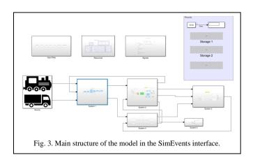
As the entity representing the treated object advances in the process, different events occur and trigger another subsystems and elements like resources. The propagation of the entities through the system is governed by a set of rules controlling the flow e.g., an entity cannot move forward if the next workstation is occupied etc.
