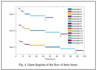
Fig. 4 shows that the flow of the objects inside the installation is continuous and in order. This shows that the flow is controlled meaning that the entity (object) cannot advance if the next workstation is occupied by treating another object.
