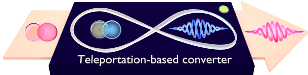
FIG. 1: An optical encoding converter for quantum interconnects. A discrete-variable qubit encoded in the Fock-state basis |\psi\rangle_{DV} = c_0|0\rangle + c_1e^{i\theta}|1\rangle is converted to a continuous-variable qubit encoded in the cat-state basis |\psi\rangle_{CV} = c_0|cat+\rangle + c_1e^{i\theta}|cat-\rangle . The heralded and postselection-free process is based on quantum teleportation via optical hybrid entanglement. The converter enables the exchange of the encoding basis while preserving the superposition, thereby allowing quantum data transfer between diverse systems and platforms.
