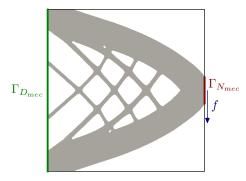
Figure 13: Shape  $\Omega_{-}$  with its boundaries and loads for the elasticity system (35).
