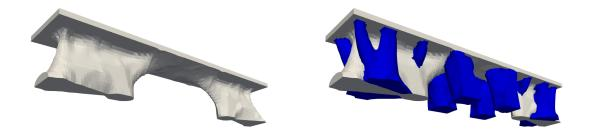
Figure 33: Problem (53): optimized shapes of the bridge  $\omega$  (white) and its supports S (blue).
