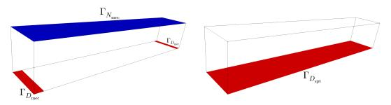
Figure 30: Boundary conditions for the mechanical equations (51) (left) and (50) (right)
