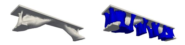
Figure 31: Problem (52): optimized shapes of the bridge  $\omega$  (white) and its supports S (blue).
