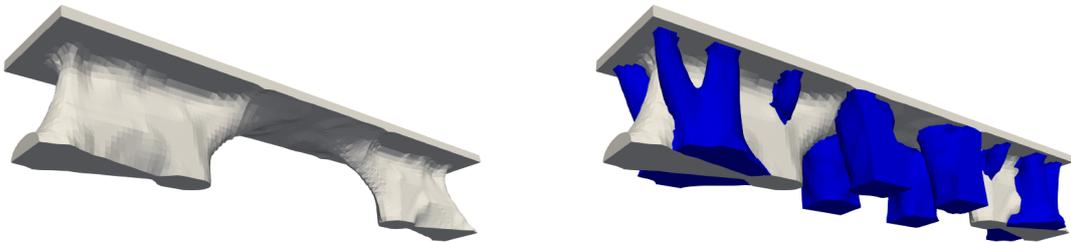
Figure 33: Problem (53): optimized shapes of the bridge  $\omega$  (white) and its supports  $S$  (blue).
