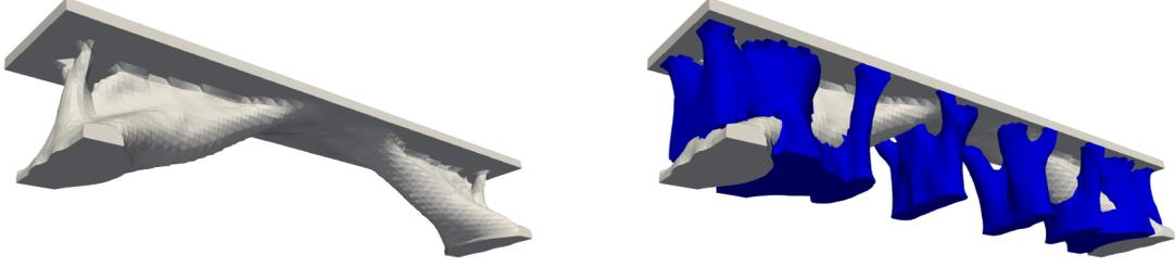
Figure 31: Problem (52): optimized shapes of the bridge  $\omega$  (white) and its supports  $S$  (blue).
