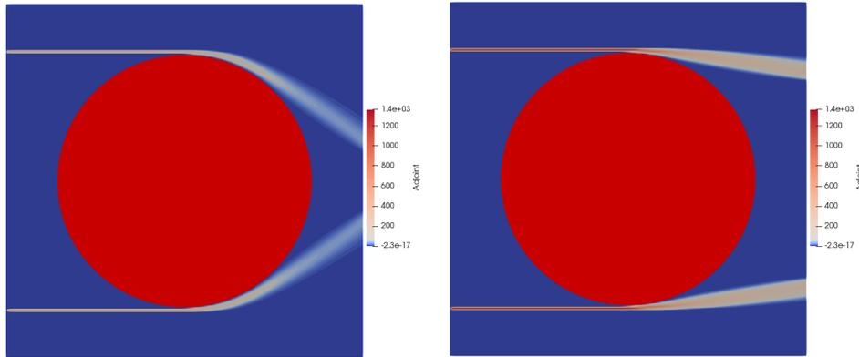
Figure 10: Adjoint state  $p$ , solution of (20) for a circular obstacle and  $J_1(\Sigma)$  (left) or  $J_{1,\varepsilon}(\Sigma)$  (right).
