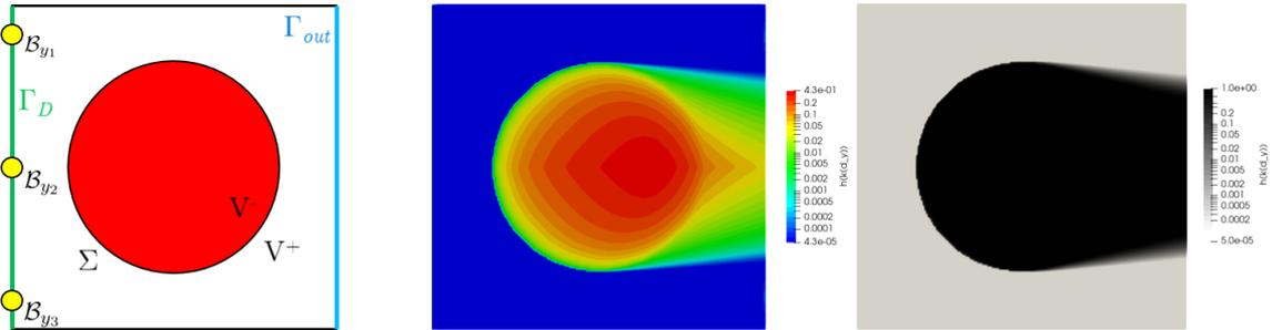
Figure 9: Accessibility of  $\Gamma_{\text{out}}$ , measured from three points on  $\Gamma_D$ , with a red obstacle (left): fields  $\min_{i=1,2,3}(d_{y_i} - d_{0,y_i})$  (middle) and  $h_\varepsilon \left( \min_{i=1,2,3}(d_{y_i} - d_{0,y_i}) \right)$  (right).
