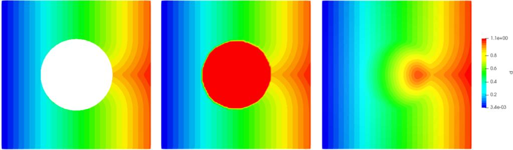
Figure 7: Solution of (7) computed in  $\Omega_+$  only (left), in the complete domain  $\Omega$  with  $V_- = 0.001$  (middle) and with  $V_- = 0.1$  (right). In all cases  $V_+ = 1$ .
