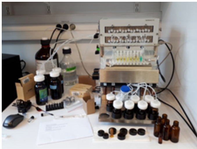
Figure 5: DNA synthesizer used for solid-phase synthesis of DNA and RNA oligonucleotides.
