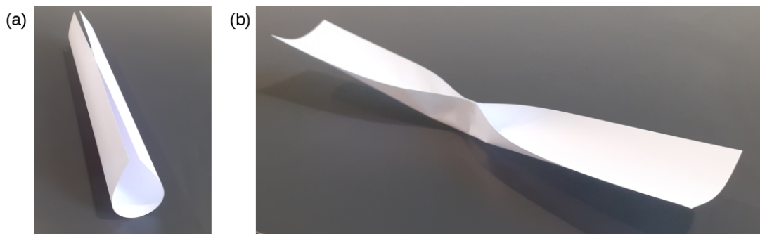
Figure 1. (a) Photograph of a rectangular paper strip ( L = 29.7 cm, W = 15 cm, t = 0.1 mm) with mid-length points at contact and maintained by an adhesive strip. (b) Photograph for a strip with a smaller width ( L = 29.7 cm, W = 5 cm, t = 0.1 mm).
